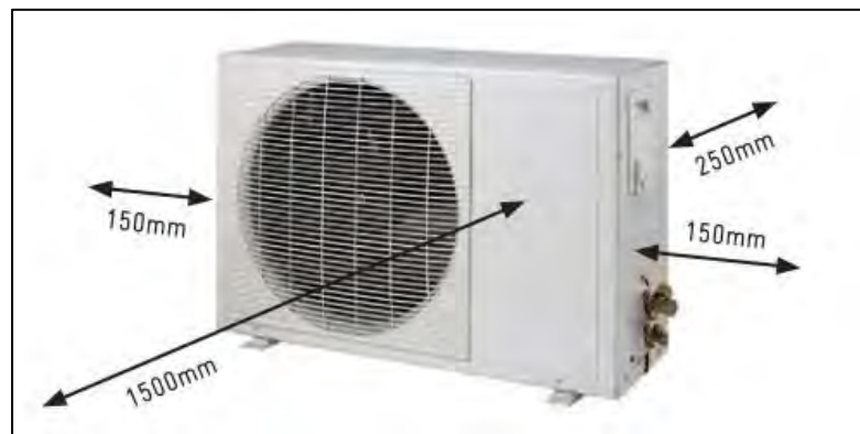
Figure 2.2: Proper location for outdoor unit
