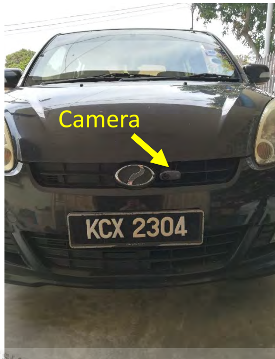
Figure 3.2: Camera mounted in front of the car
