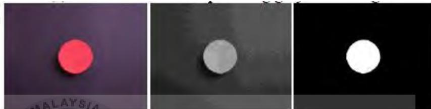
Figure 2.1: Otsu's threshold output using lightness channel [1]
