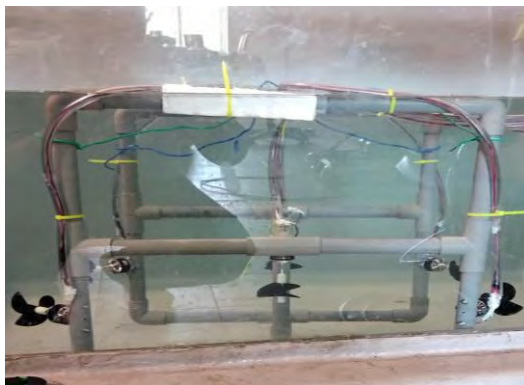
Figure 4.13: Balancing test of ROV.
