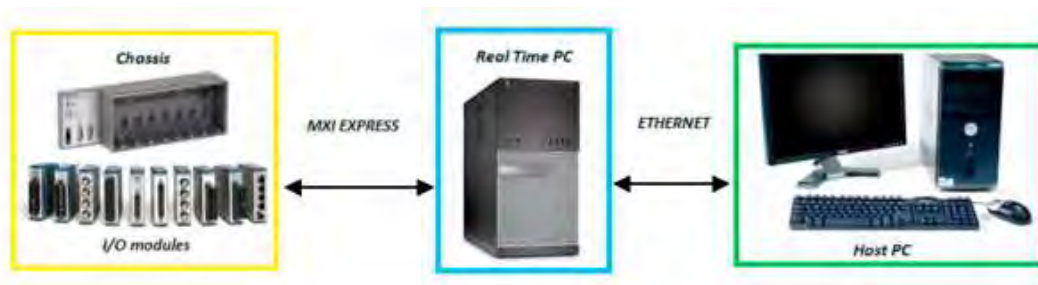
Figure 2.3 Control system structure
