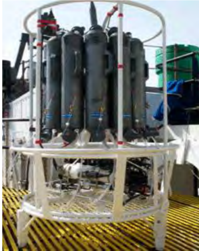
Figure 1: Rosette Sample that utilized to gather samples of water in ocean
