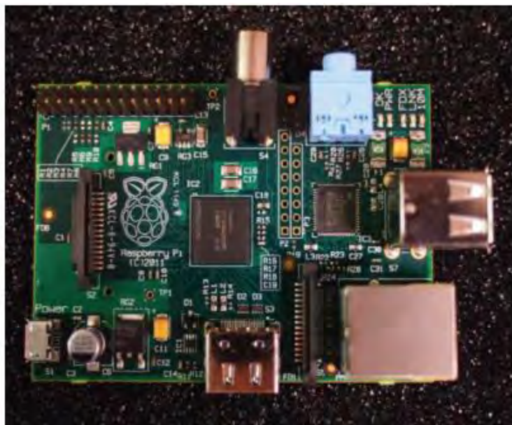
Figure 2.3 Raspberry Pi Board Representation[17]
