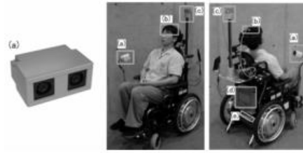
Figure 2.2: A stereo camera and experimental system (Yoda et al., 2013)
