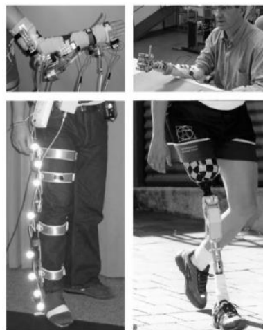
Figure 1.12 Wearable Robots (2): (top and bottom left) orthotic exoskeletons; (top and bottom right) prosthetic robot.
