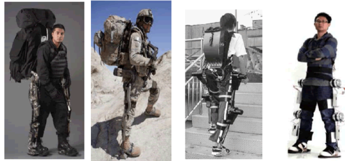
Figure 1.11 Wearable Robots (1): lower limb empowering robotic exoskeleton.
