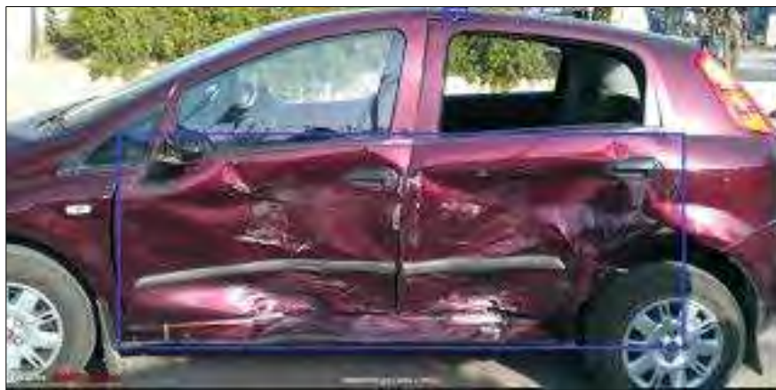
Figure 2.1: Vehicle door panel deformation after crash. Source:
