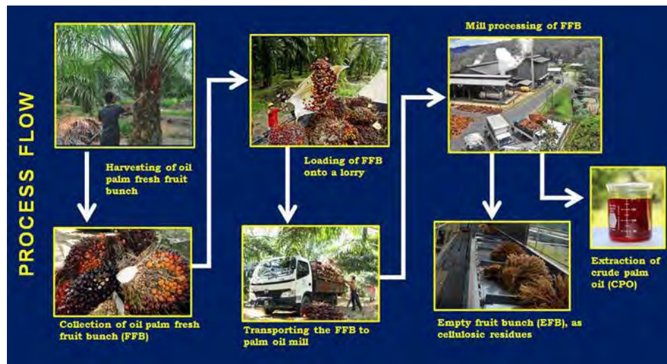
Figure 1.3: The palm oil process flow
