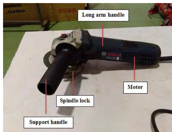
Figure 1.1: Main components of hand grinder
