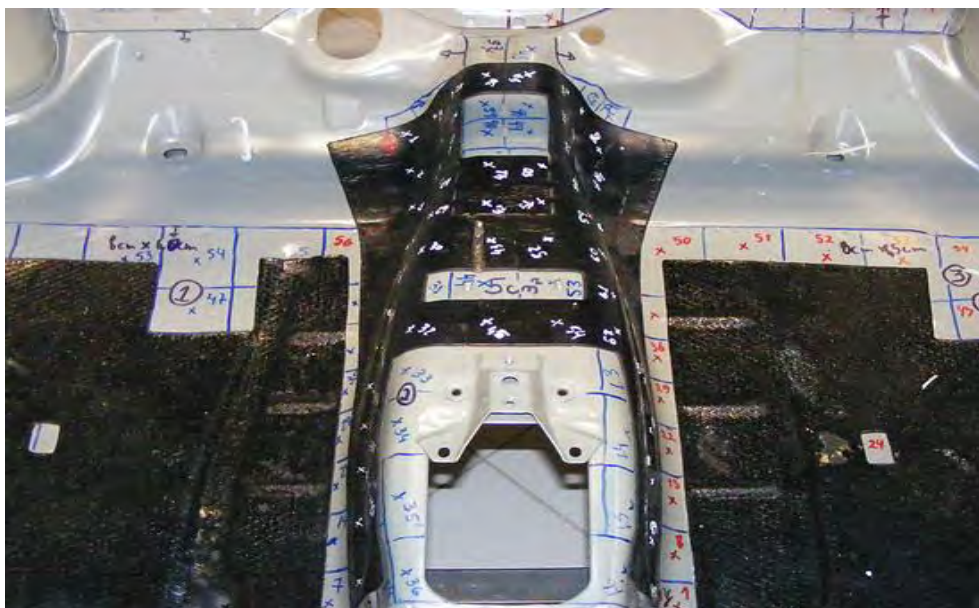
Figure 1.1: Damping material applied on body panels
