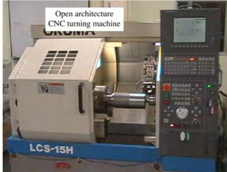
Figure 2.2: Open architecture CNC turning machine employed for experiments
