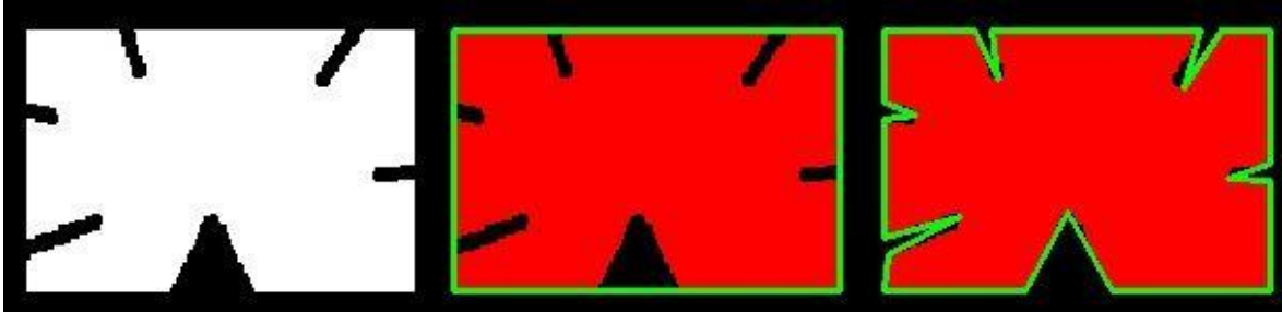
Figure 3.17: Original image, image with 10% epsilon and image with 1% epsilon ( https://docs.opencv.org/3.4/dd/d49/tutorial_py_contour_features.html )
