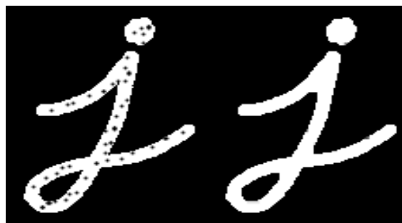
Figure 3.15: Closing morphological operation ( https://docs.opencv.org/3.4/d9/d61/tutorial_py_morphological_ops.html )
