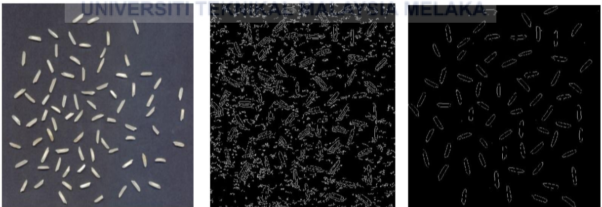
Figure 2.15: Process to determine the chalky in the grain (rice) (Parveen, 2017).
