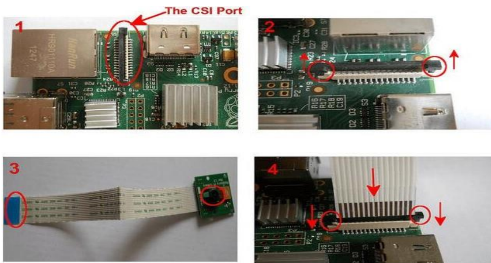
Figure 3.6: Picamera installation guide (Nora, 22 nd Dec 2016)
