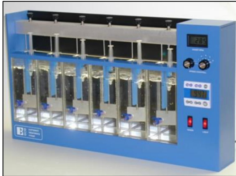
Figure 2.1: The Jar Test Machine. Taken from “Coagulation and Flocculation.” Introduction to Potable Water Treatment Processes , Mar. 2009, pp. 26–42., doi:10.1002/9781444305470.ch3.[3]
