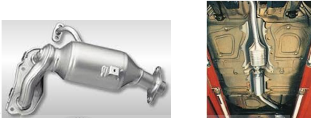
Figure 2.2: Close-coupled Catalytic Converter (Left) and Underfloor Catalytic Converter (Right)
