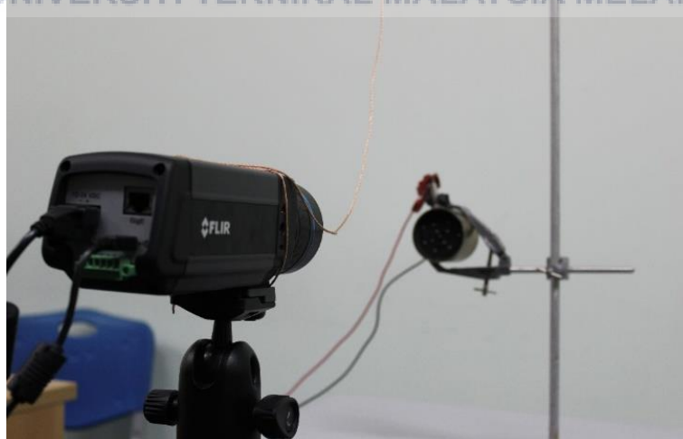
Figure 3.2: thermographic camera must be aligned parallel with EHC
