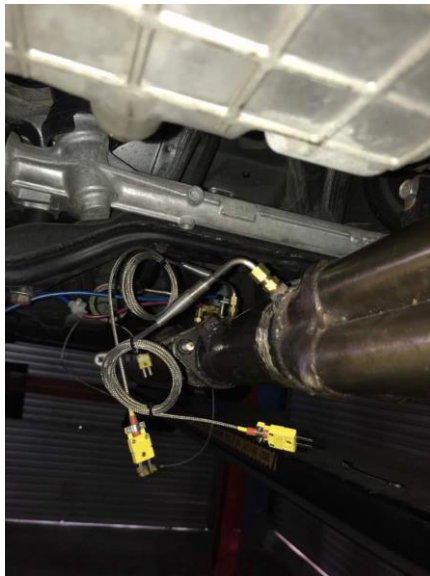
Figure 3.8: Thermocouples are fitted into exhaust (left) and data logger system (right)
