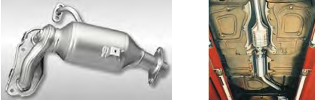
Figure 2.2: Close-coupled Catalytic Converter (Left) and Underfloor Catalytic Converter (Right)
