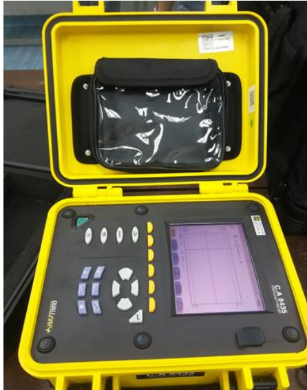
Figure 3.23: Chauvin Arnoux C.A 8435 energy meter
