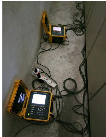
Figure 3.24: Measurement using two Chauvin Arnoux C.A 8435
