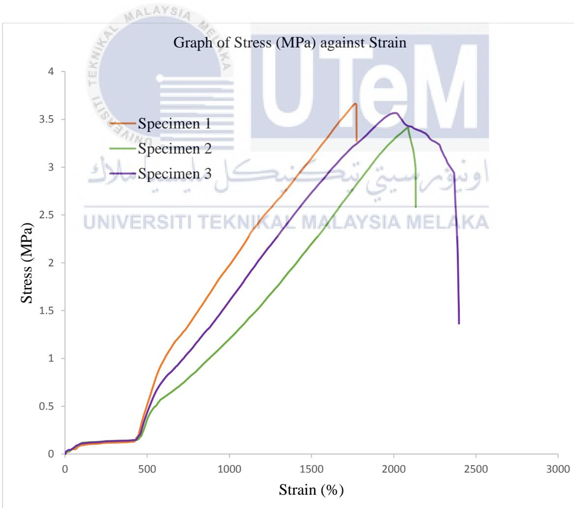
Figure 4.20: Graph of stress against strain of joints bonded for humidity test at 85°C/40RH (3 days)
