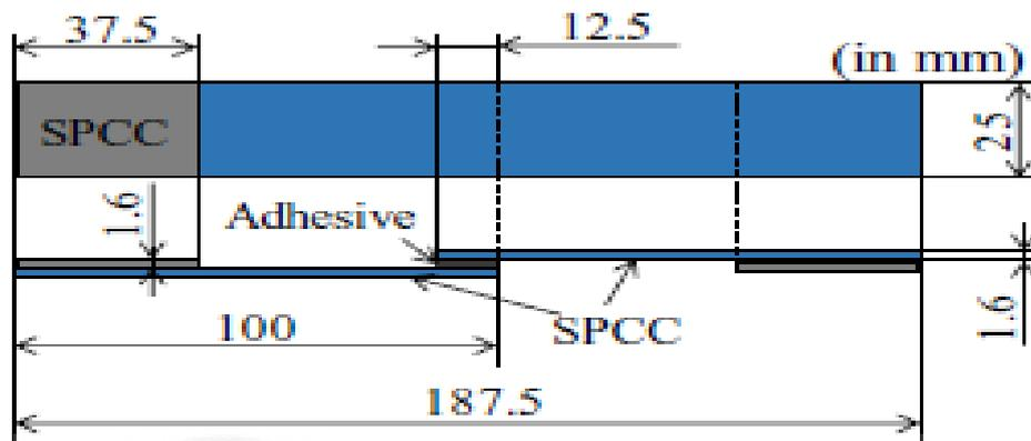
Figure 2.3: Shape and dimension of lap joint specimen [23]
