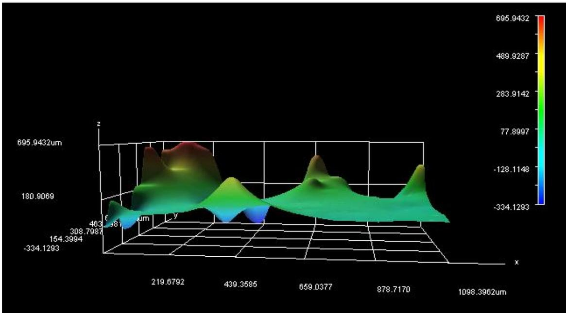
Figure 4.12: Surface topography after lap shear tensile test of joints bonded for humidity test at 85°C/85RH (1 day)
