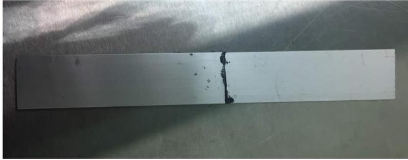
Figure 3.17: Sample of specimen after bonding and curing process at room temperature
