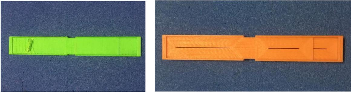
Figure 4.2: Second prototypes of jig with improper surface finish and presence of gap
