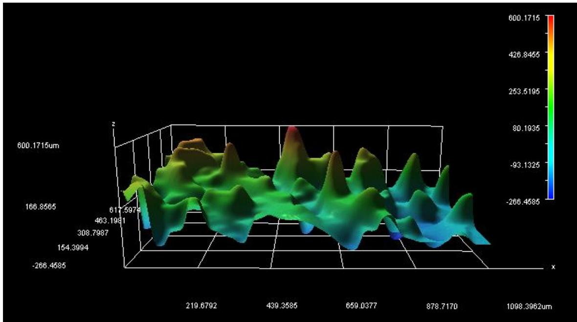
Figure 4.10: Surface topography after lap shear tensile test at room temperature
