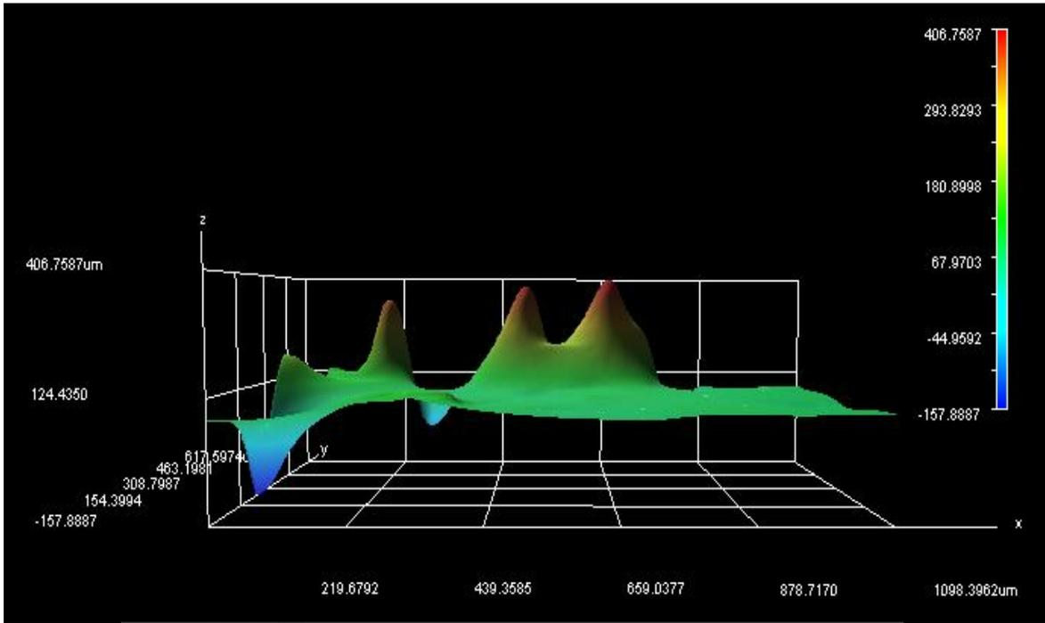
Figure 4.19: Surface topography after lap shear tensile test of joints bonded for humidity test at 85°C/40RH (1 day)
