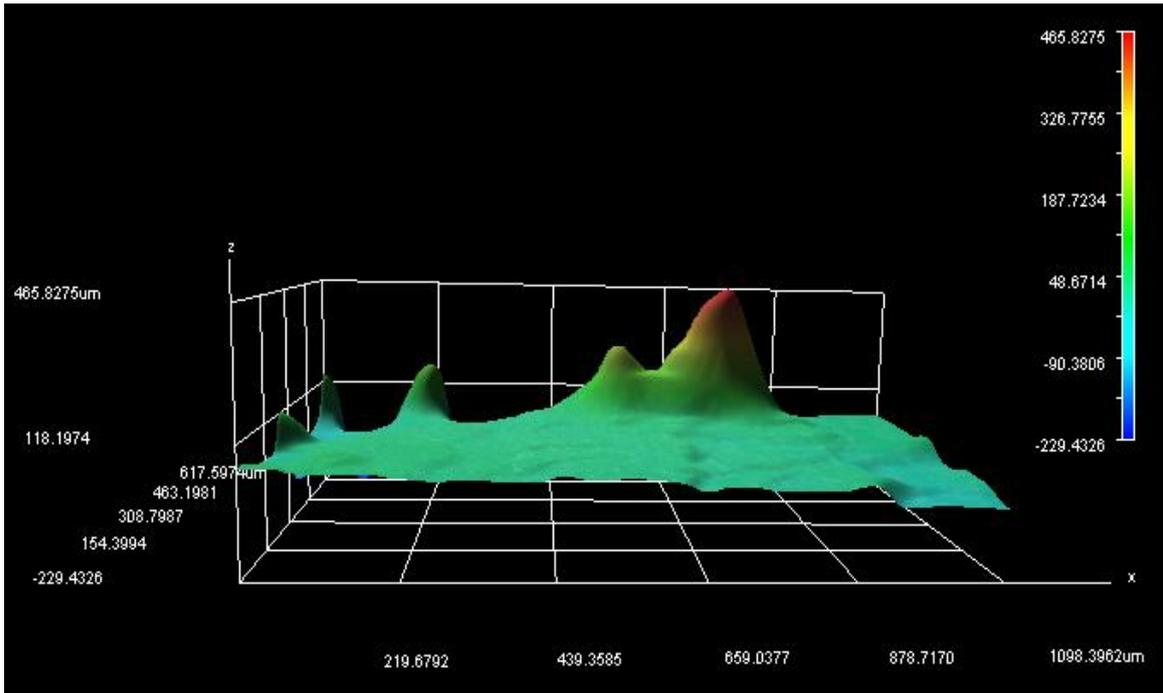
Figure 4.21: Surface topography after lap shear tensile test of joints bonded for humidity test at 85°C/40RH (3 days)
