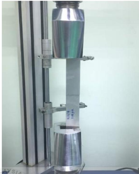
Figure 3.24: Specimen with tensile grips
