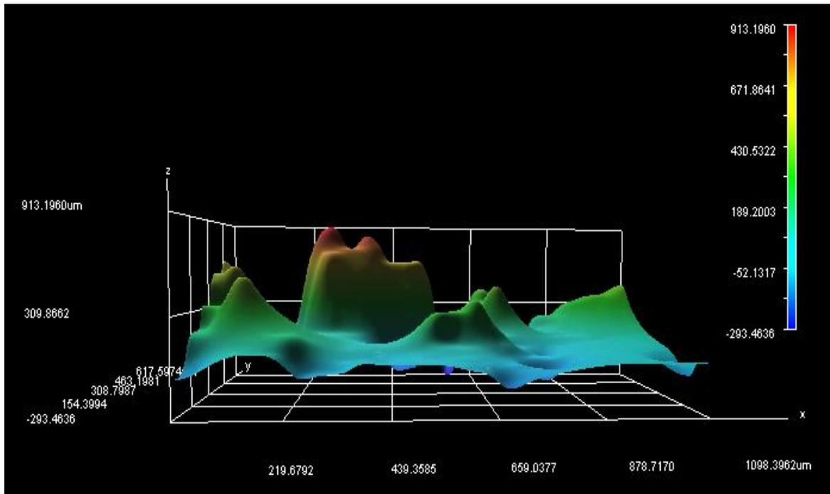
Figure 4.16: Surface topography after lap shear tensile test of joints bonded for humidity test at 85°C/85RH (5 days)
