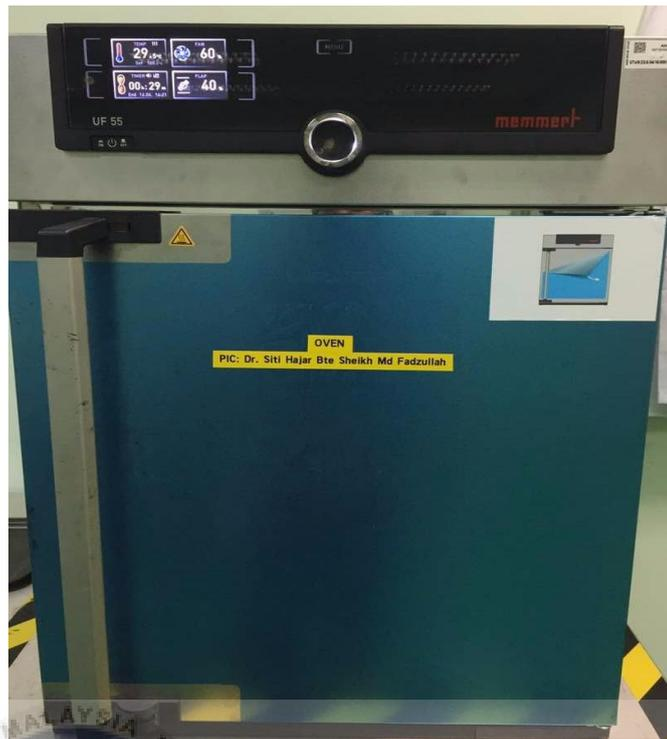
Figure 3.19: Specimens were heated in the oven with temperature of 100°C within 30 minutes
