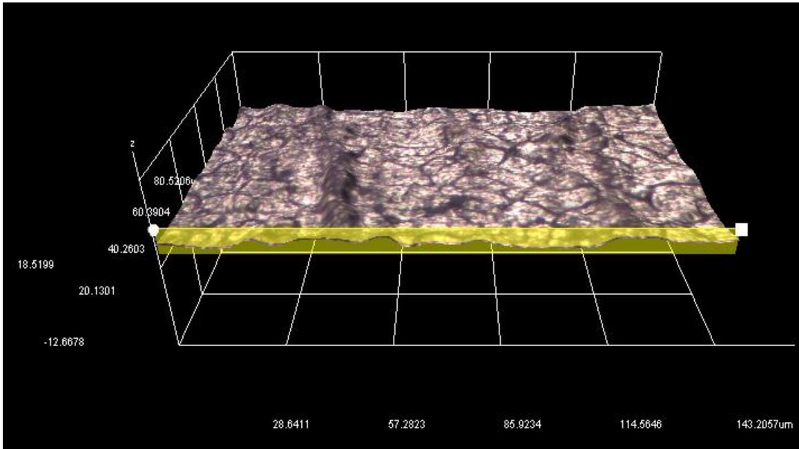
Figure 4.8: Surface 3D profile with surface treatment before adhesively bonded process
