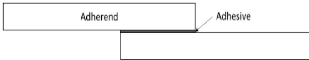
Figure 2.1: Single lap (unsupported) joint [7]
