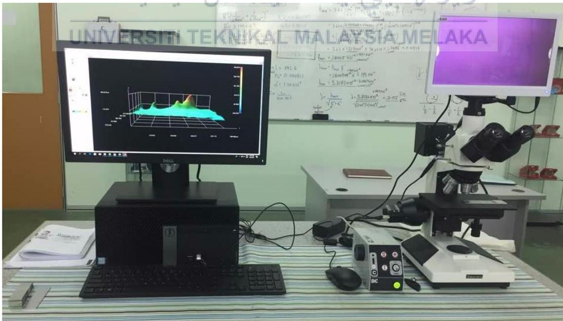
Figure 3.26: Surface profiling under 3D non-contact surface profilometer
