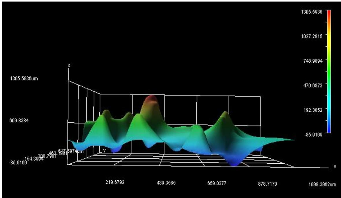
Figure 4.14: Surface topography after lap shear tensile test of joints bonded for humidity test at 85°C/85RH (3 days)
