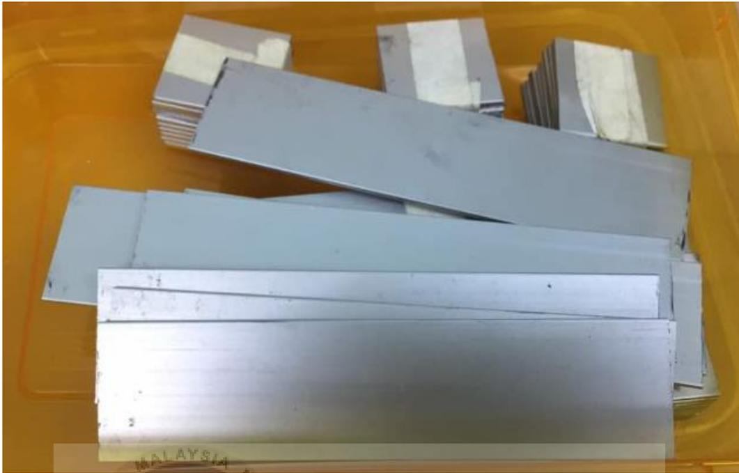
Figure 3.8: Sample of test specimens and grips
