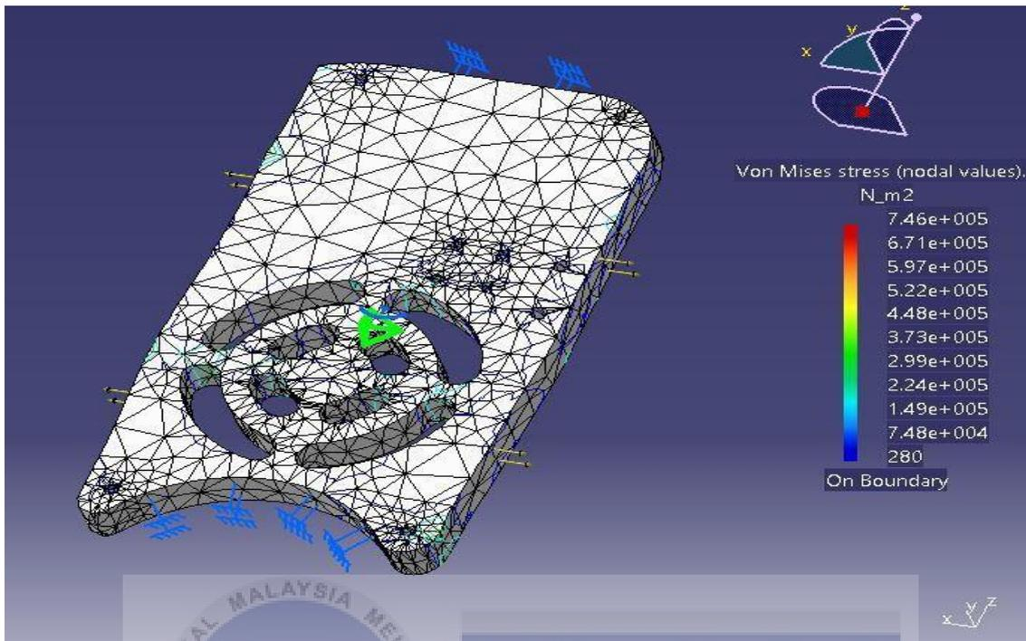
Figure 27 Front panel 100N force tension
