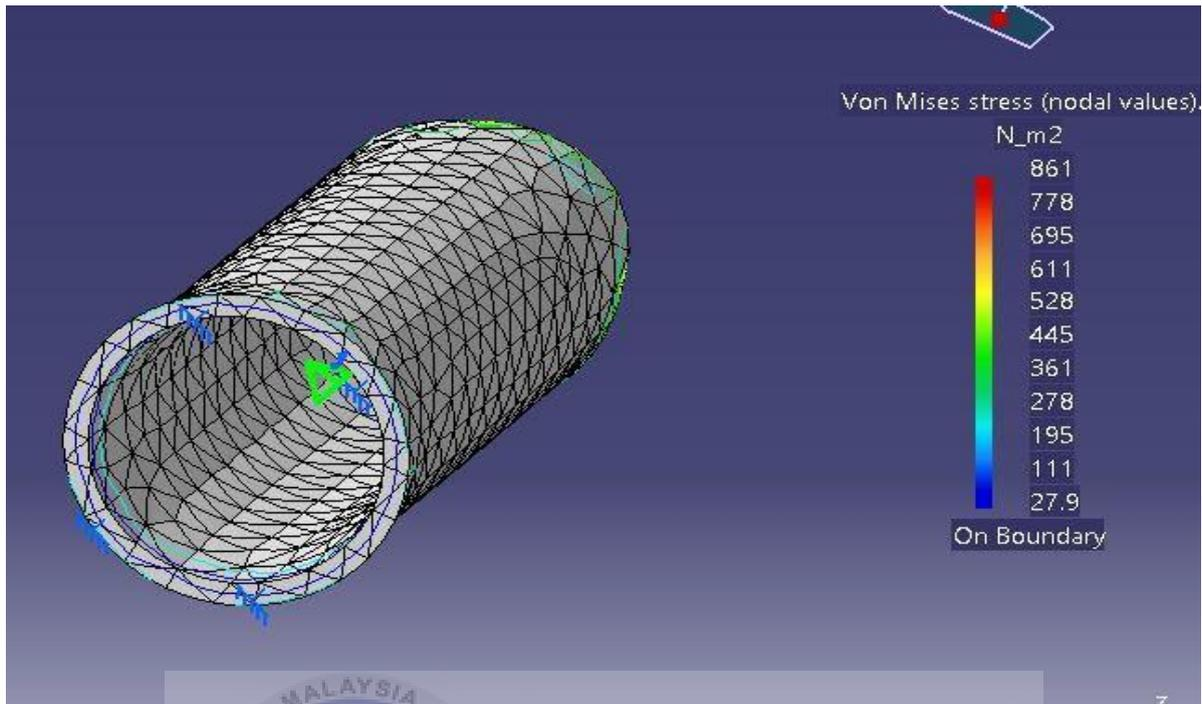
Figure 41 Middle cylinder body 100N force tension
