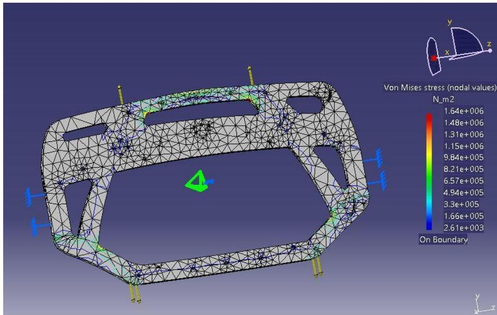
Figure 36 Side body 100N force tension
