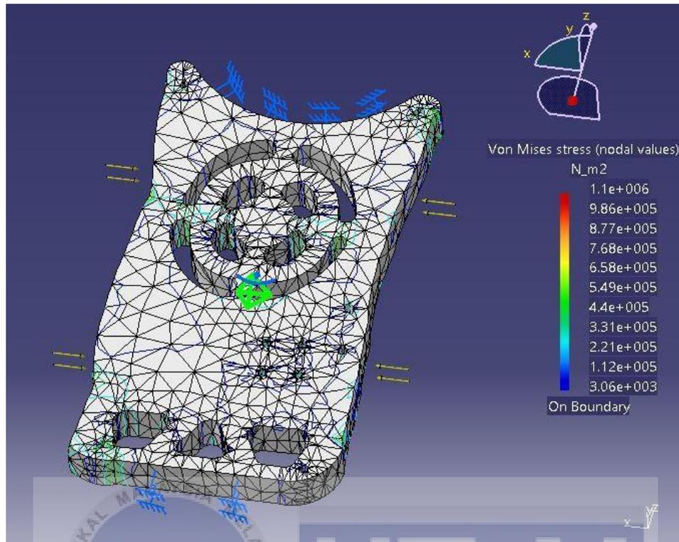
Figure 23 Rear panel 200N force compression
