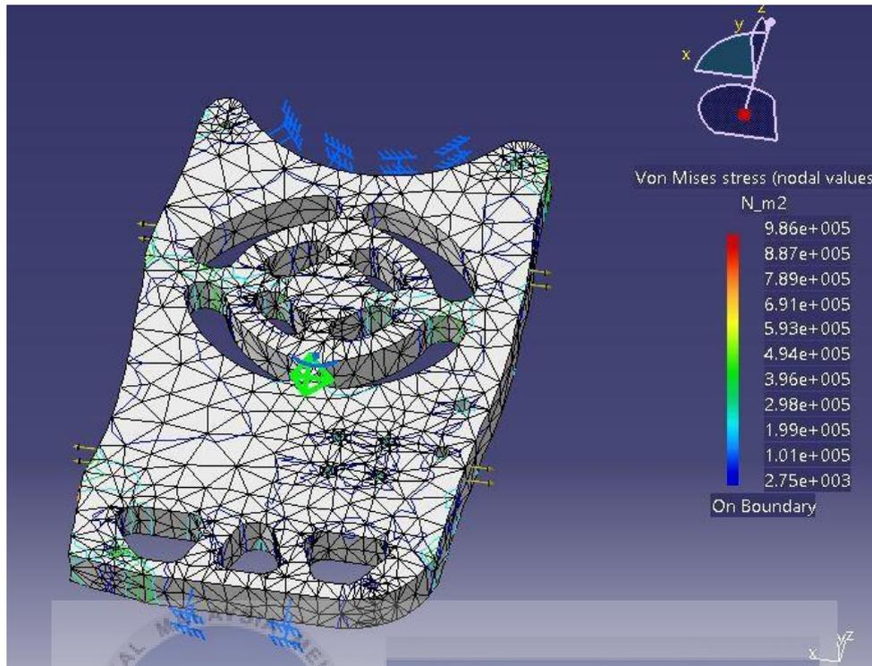
Figure 21 Rear panel 180N Tension
