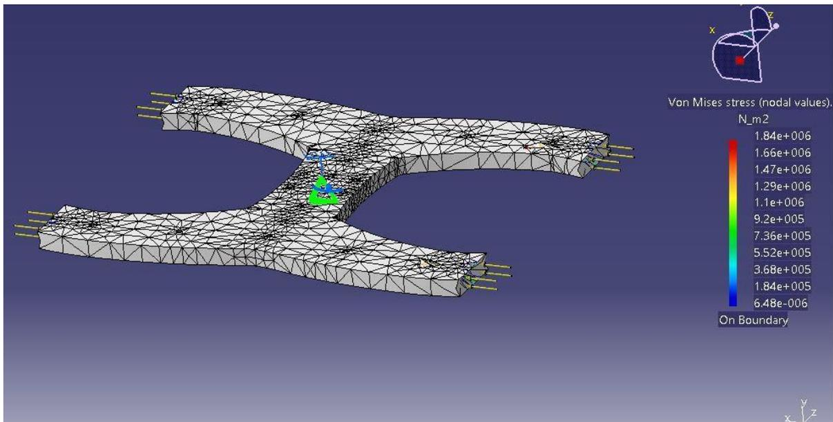
Figure 17 Bottom Body 200N force Compression
