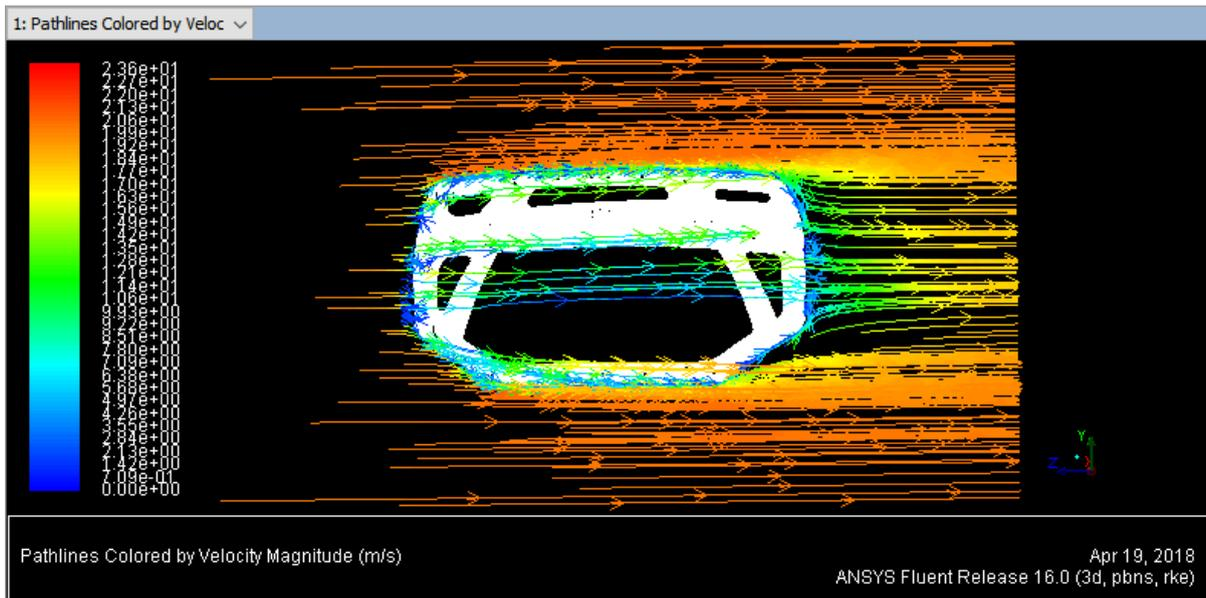
Figure 47 Side body (front flow)
