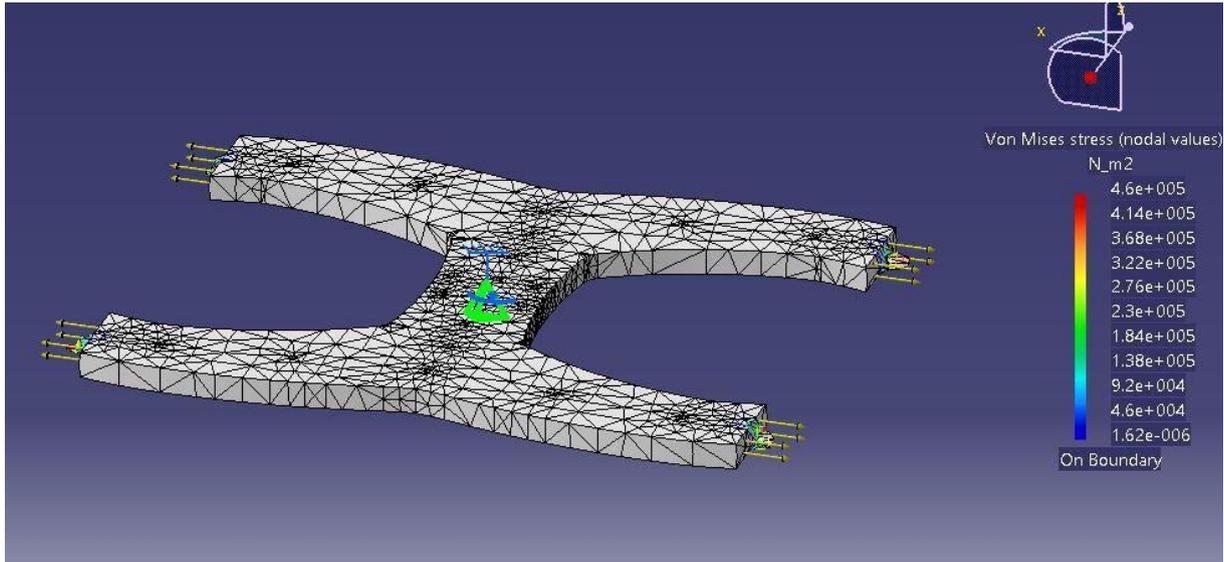
Figure 19 Bottom Body 50N force Tension
