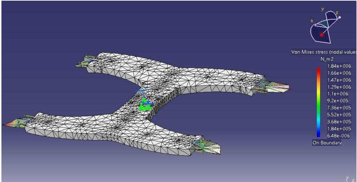
Figure 18 Bottom Body 200N force Tension
