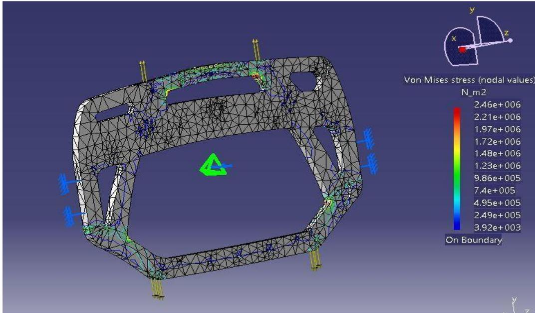
Figure 35 Side body 150N force tension
