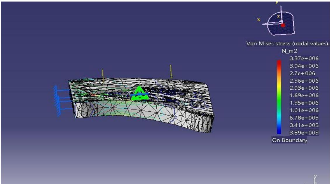
Figure 33 Front panel 300N force bending
