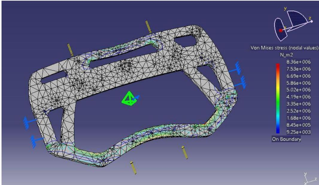
Figure 37 Side body 300N force compression
