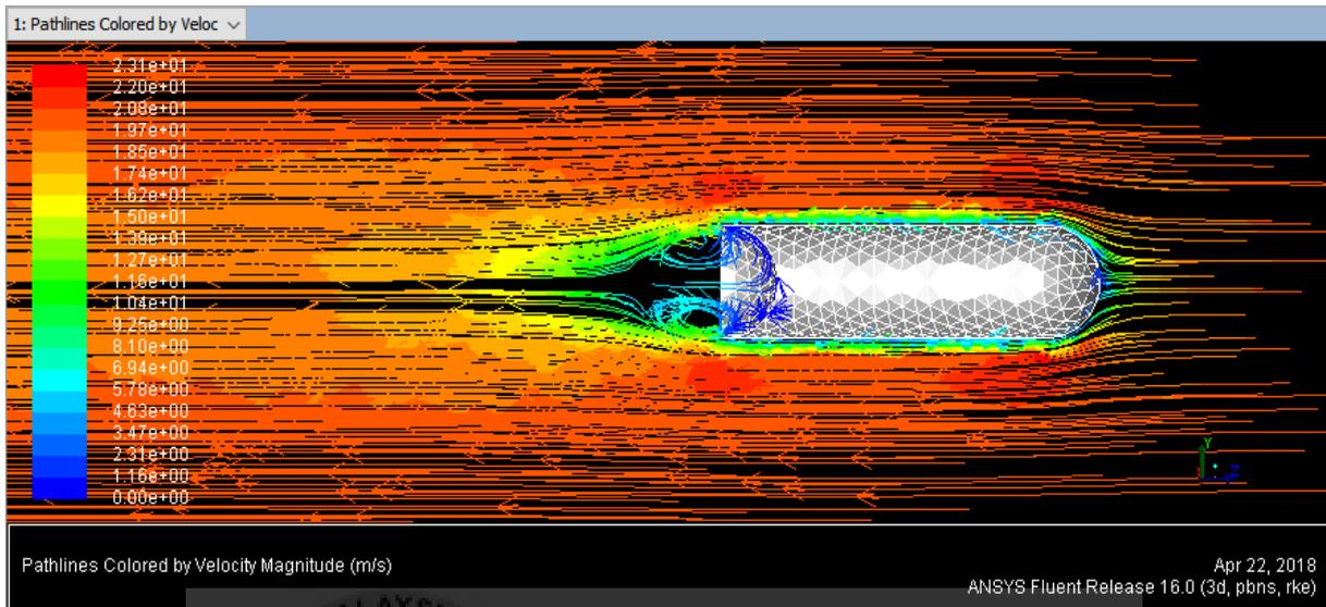
Figure 50 Middle cylinder body (front flow)
