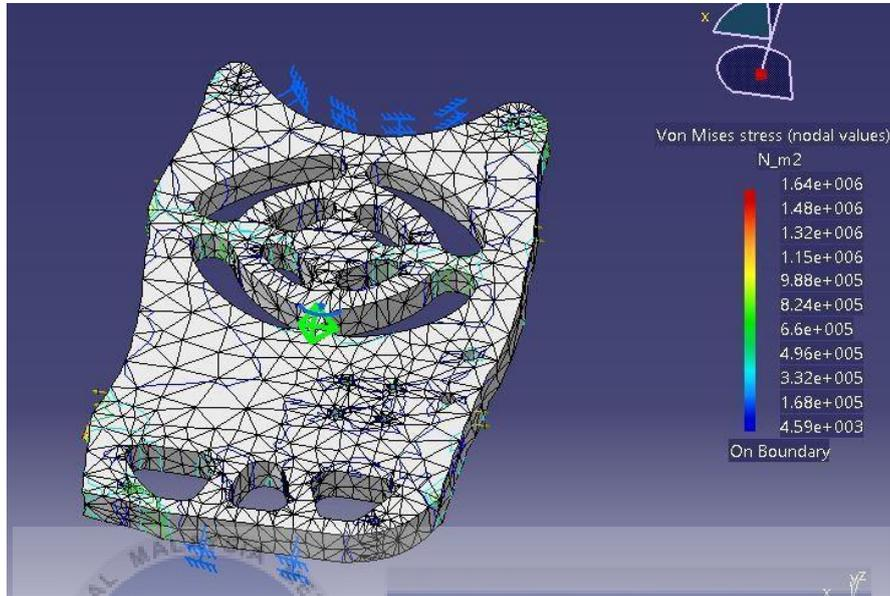
Figure 20 Rear Panel 300N Force tension
