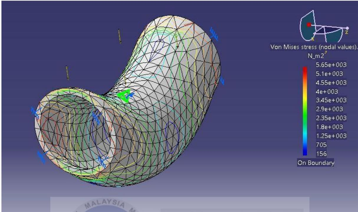
Figure 44 Middle cylinder body 50N force load
