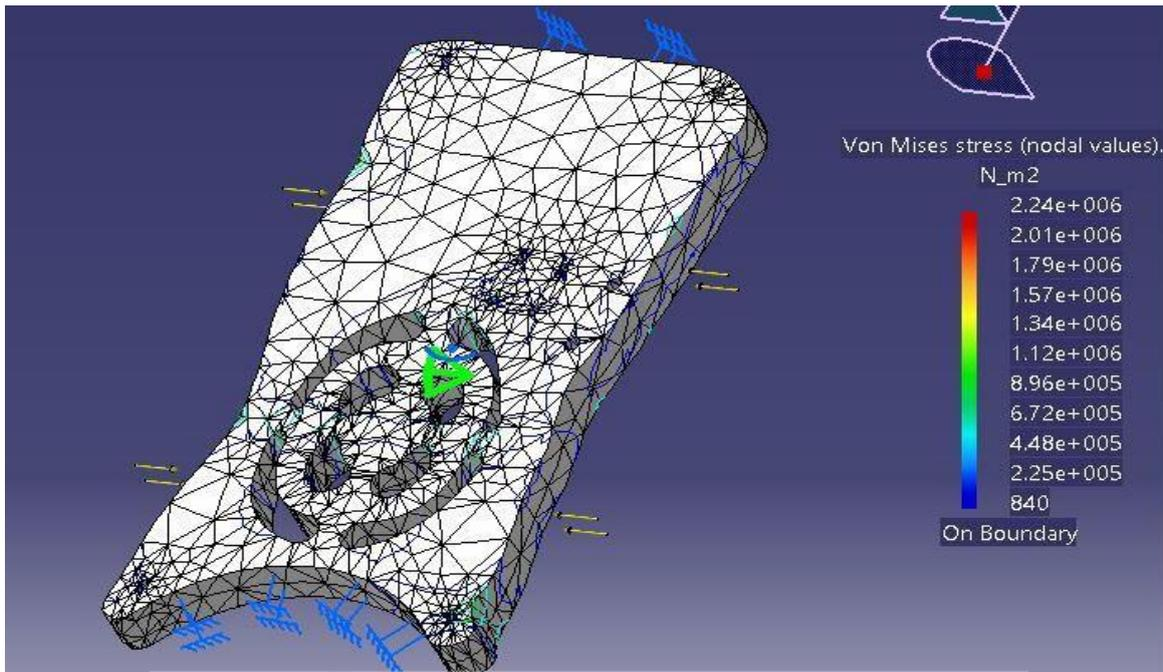
Figure 30 Front panel 300N compression
