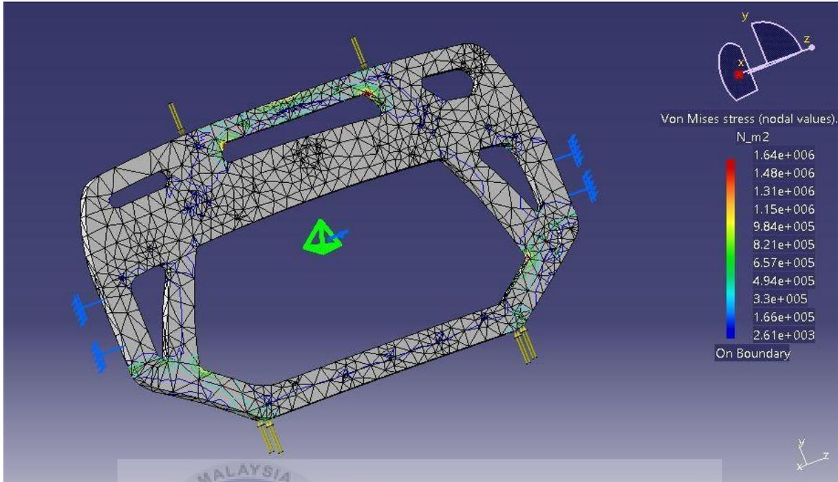
Figure 39 Side body 100N force compression
