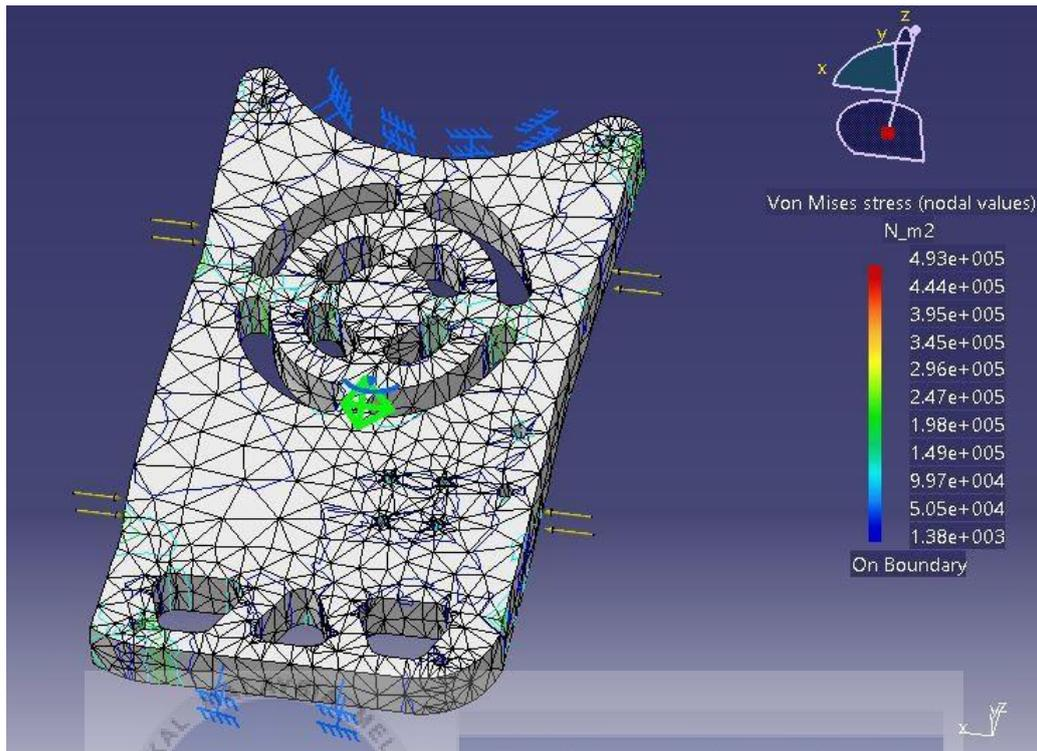
Figure 24 Rear panel 90N force compression
