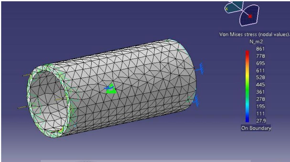
Figure 43 Middle cylinder body 100N force compression
