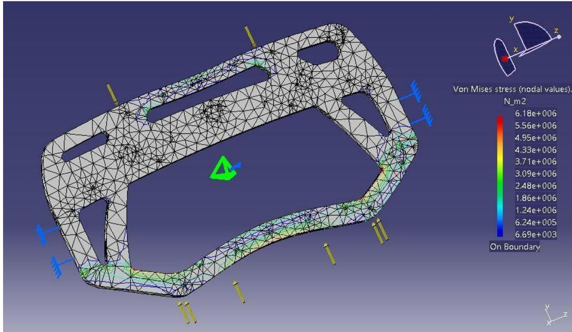
Figure 38 Side body 200N force compression
