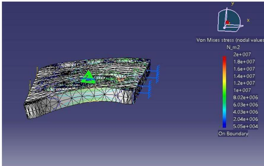
Figure 25 Rear Panel 300N Force bending
