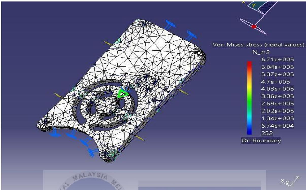
Figure 32 Front panel 90N force compression
