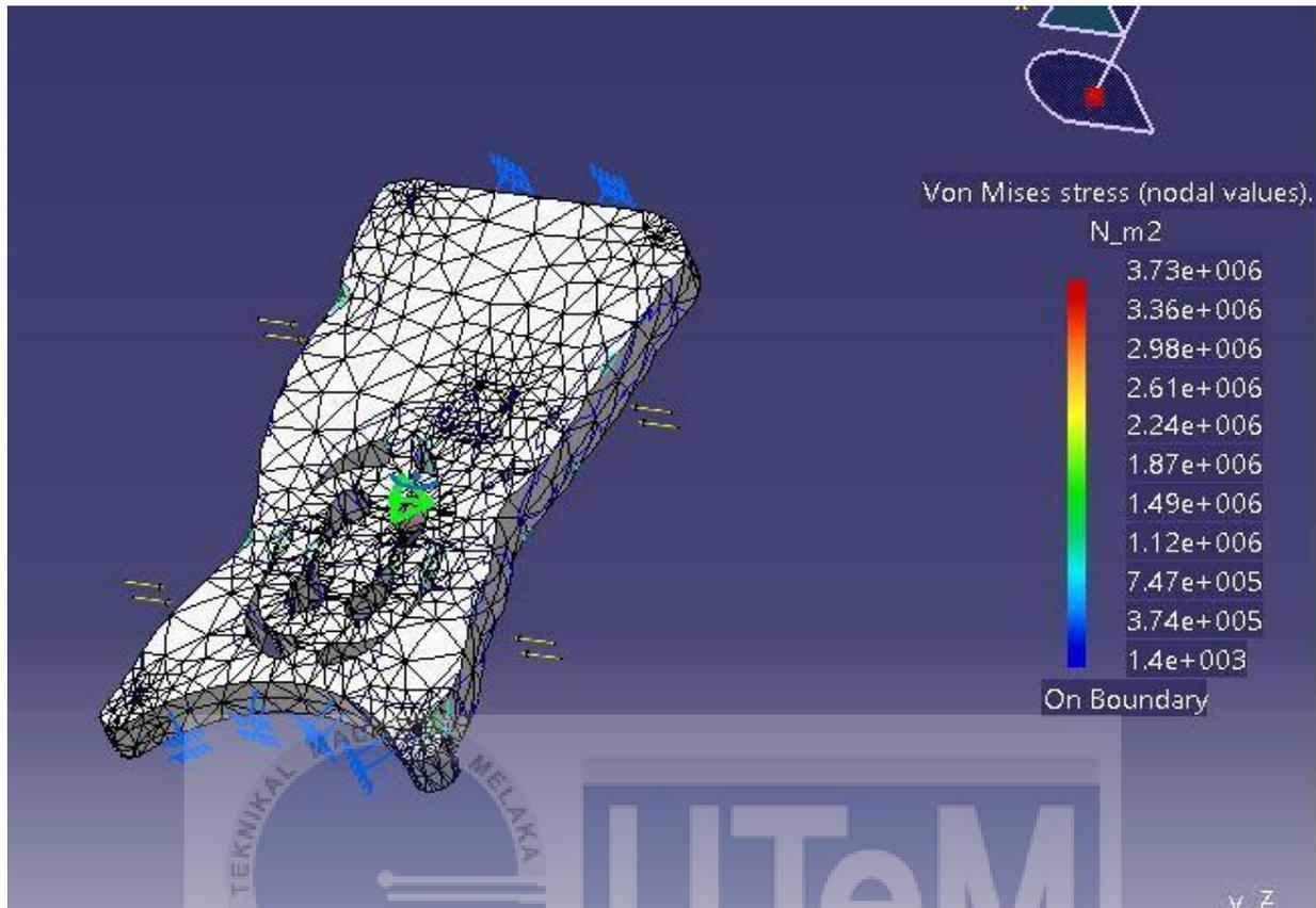
Figure 29 Front panel 500N force compression
