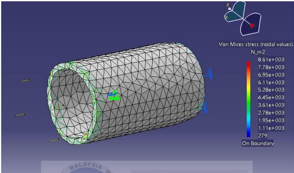
Figure 42 Middle cylinder body 500N force compression
