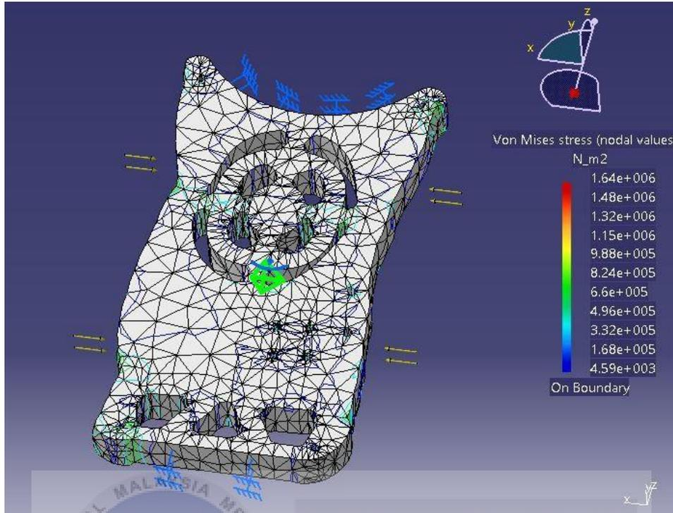
Figure 22 Rear panel 300N force compression
