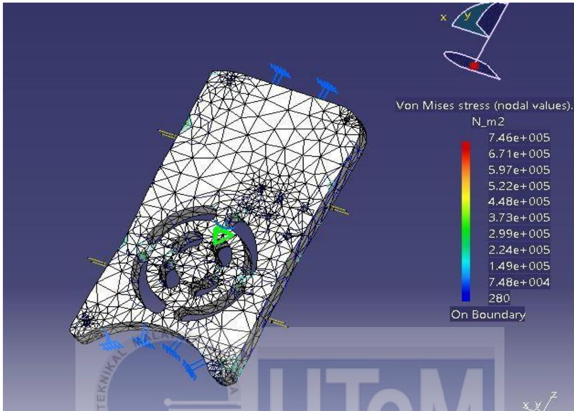
Figure 31 Front panel 100N compression
