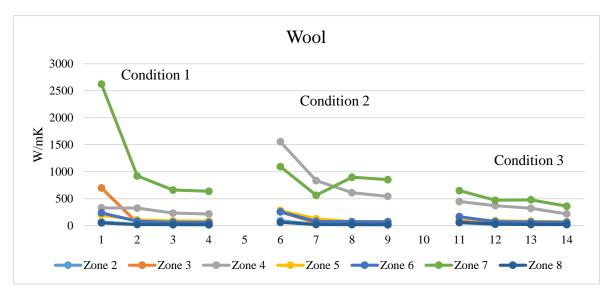
Figure 5.4: Wool insulations tested under different conditions.
