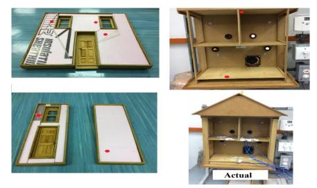
Figure 4.9: Locations (red dots) of thermocouples will be installed.
