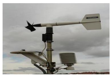
Figure 3.5: Weather station to monitor the weather conditions.
