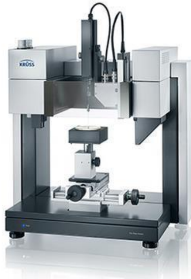
Figure 2.9: Drop Shape Analyzer – DSA100
