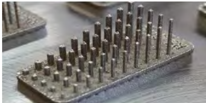
Figure 2.4: Fabricated struts with different diameters.
