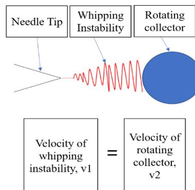
Figure 4.8: Schematic drawing of whipping instability during process electrospinning
