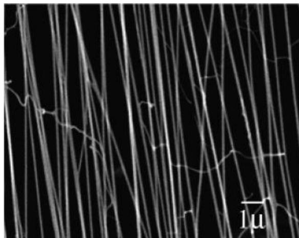
Figure 1.2 : Aligned nanofiber (Katta *et al.*, 2004)
