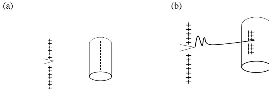
Figure 4.6: Schematic diagram of residual charge effect (a) before electrospinning process (b) during electrospinning process
