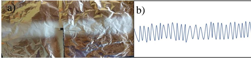
Figure 4.4: Deposition of electrospun nanofiber on distance 10 cm (a) On aluminum foil (b) Schematic drawing on aluminum foil
