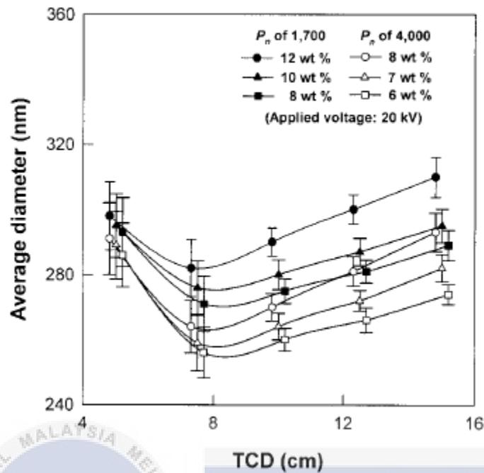
Figure 2.6: Average diameter of PVA nanofiber as function of needle tip to collector (Lee *et al.*, 2004)
