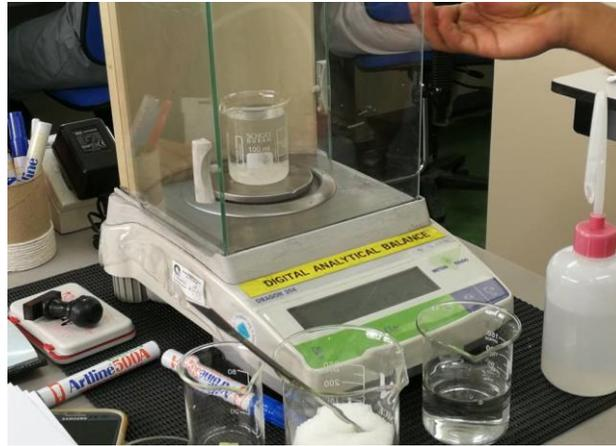
Figure 3.2: Digital Analytical Balance
