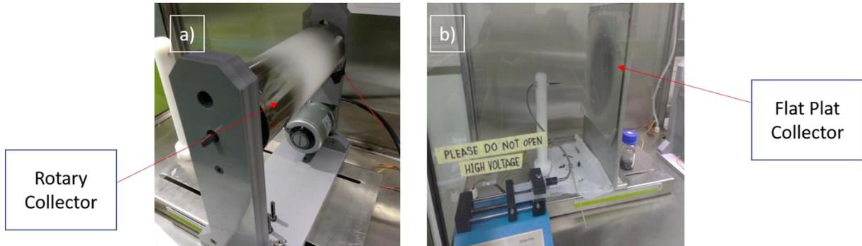
Figure 4.2: a) Rotary Collector b) Flat Plat Collector
