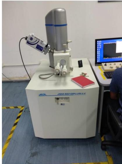
Figure 3.6: Scanning Electron Microscopy machine (JEOL JSM-6010PLUS/LV)
