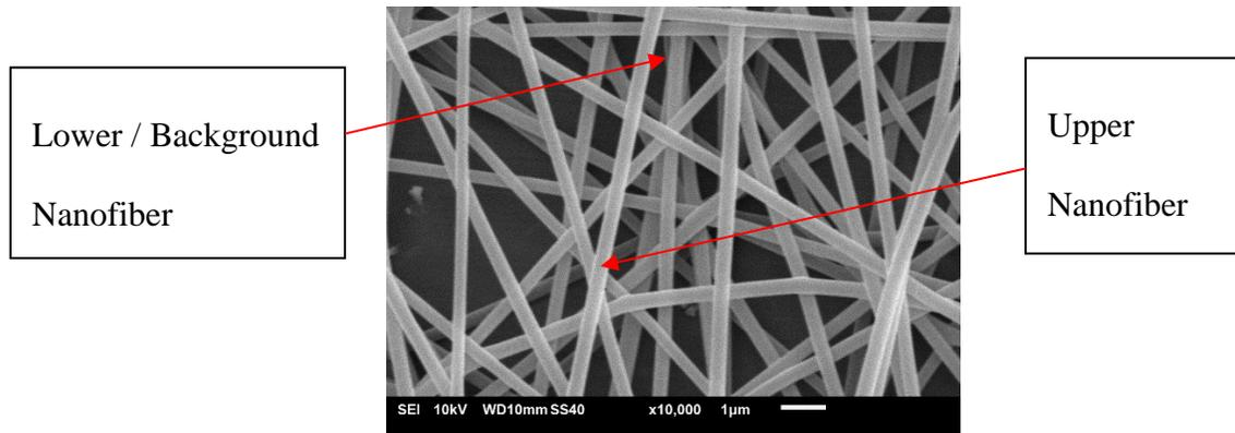
Figure 4.7: SEM micrograph on rotating collector at speed 1600 RPM
