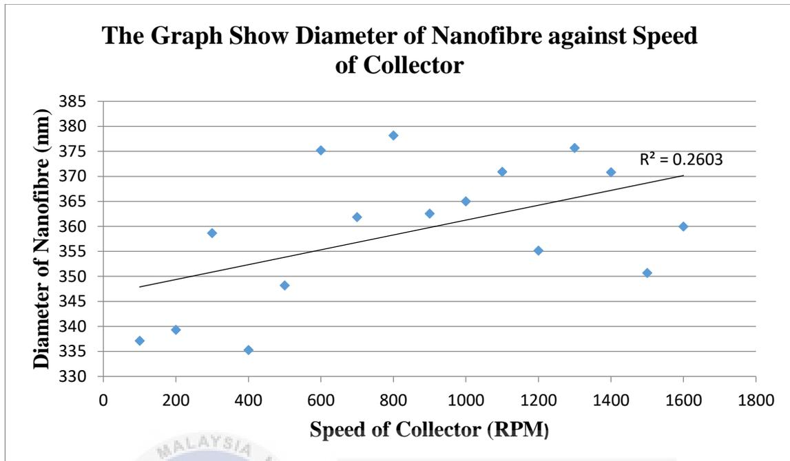
Figure 4.5: The graph shows diameter of nanofiber against speed of collector
