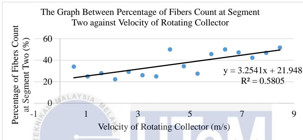
Figure 4.9: Graph show percentage of fibers count at segment two against velocity of rotating collector
