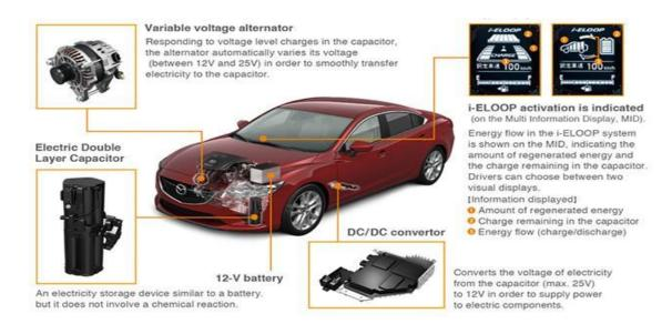
Figure 7 : Electric Double Layer Capacitor in Vehicle (Mazda, n.d)
