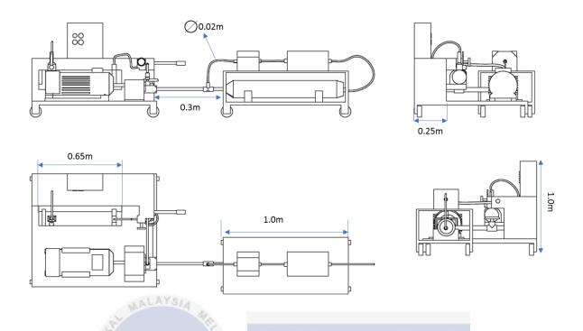
Figure 12 : Orthographic View of Test Rig
