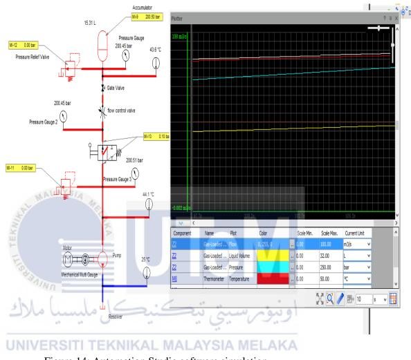
Figure 14: Automation Studio software simulation
