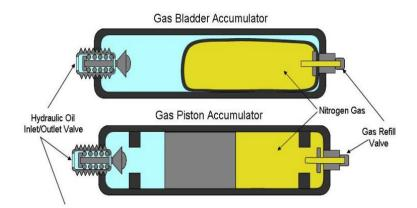
Figure 4 : Bladder and Piston Accumulator.
