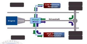
Figure 2: Component of Regenerative Braking in Hydraulic Hybrid System
