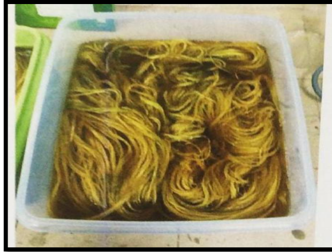
Figure 3.3: Kenaf fibre were soaked in NaOH solution
