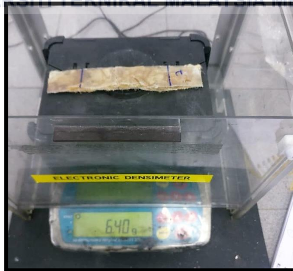
Figure 3.15: The apparent mass of Kenaf Fibre/PP composite specimen was measured
