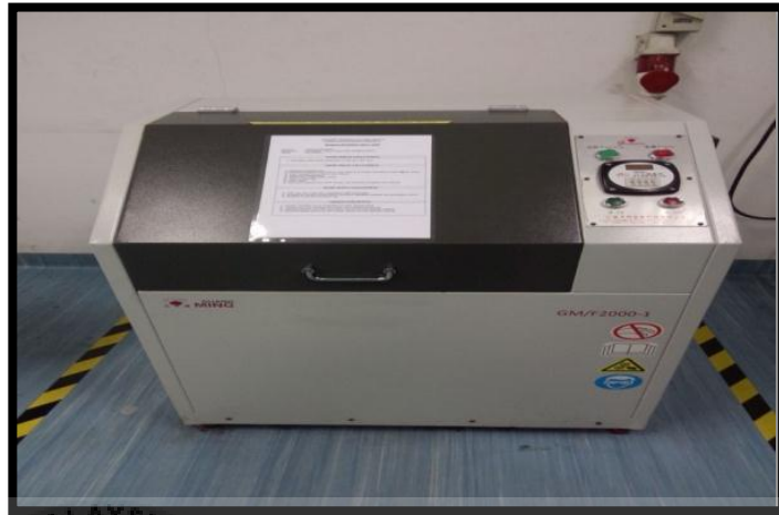
Figure 3.5: Pulverizer machine is used to crush PP
