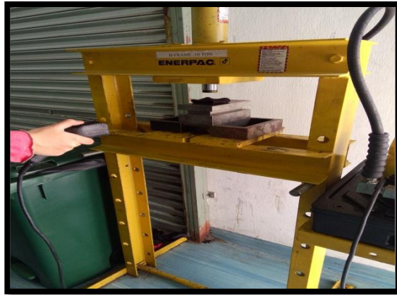
Figure 3.9: The mould opener machine
