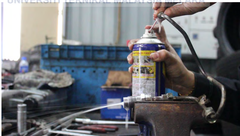
Figure 4.4.2: Spray pattern of fuel injector without nozzle needle
