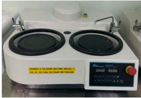
Figure 3.3: Grinder and polishing machine for substrate surface treatment.
