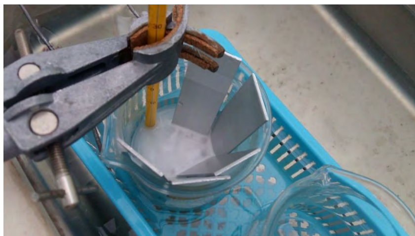
Figure 3.7: Air bubbles formed as the NaOH solution react to aluminium surface.
