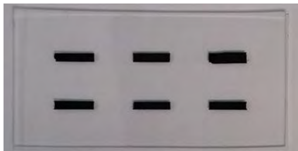
Figure 3.25: Printed ECA on polycarbonate sheet.
