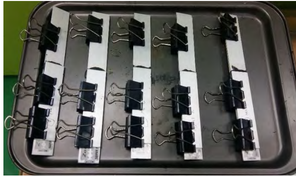
Figure 3.22: Single-lap-joint adhesively bonded samples are put into oven for ECA curing process.
