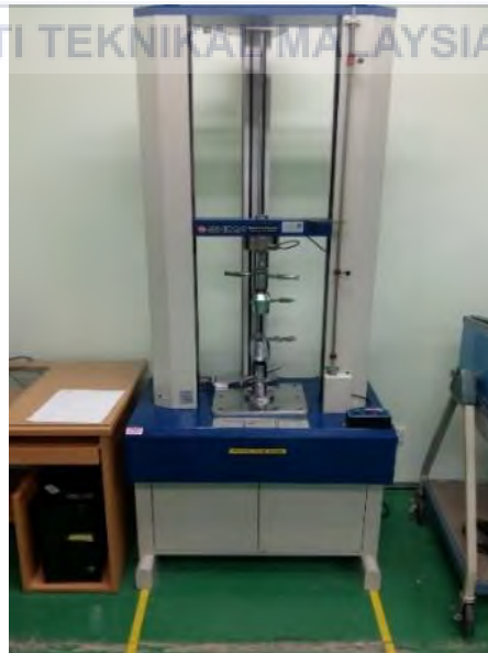
Figure 3.30: Universal Material Testing (AG-10kNX) used for lap shear test.
