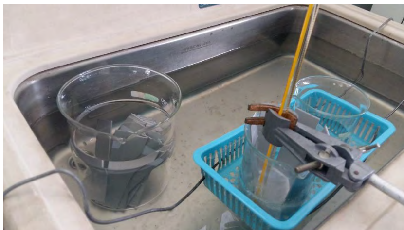
Figure 3.6: The complete set up of chemical etching process.
