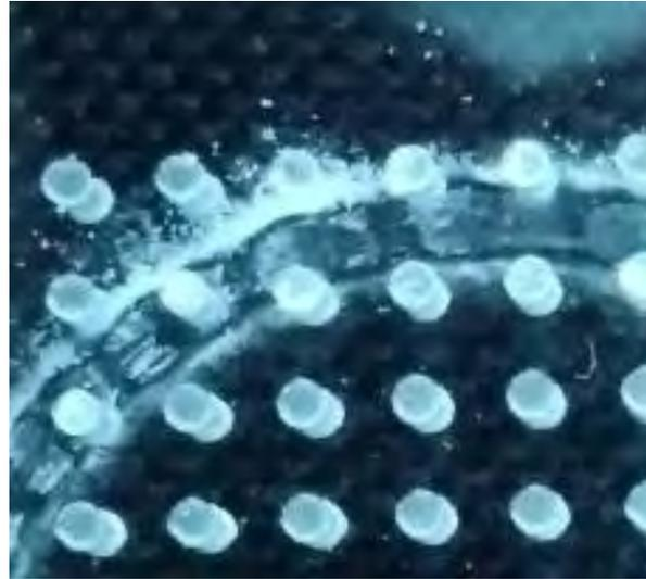
Figure 4.14: Debris along wear track for specimen B
