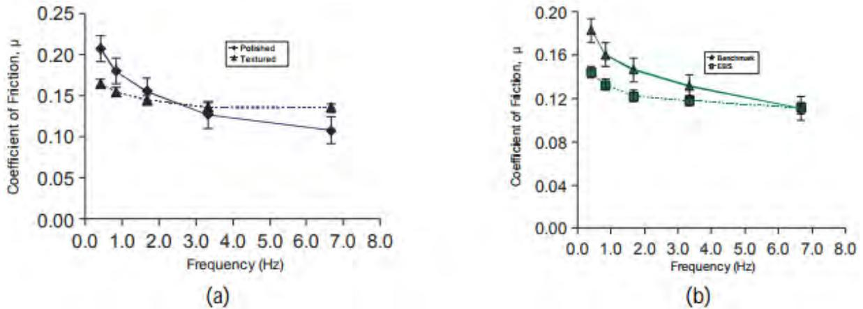
Figure 2.15: Coefficient of friction as a function of reciprocating frequency using low viscosity lubricant (Norpar-18). a) Normal load of 90 N; b) normal load of 130 N
