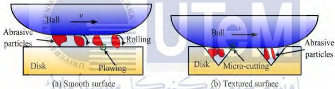
Figure 2.21: Friction and wear mechanism of the smooth and textured surface
