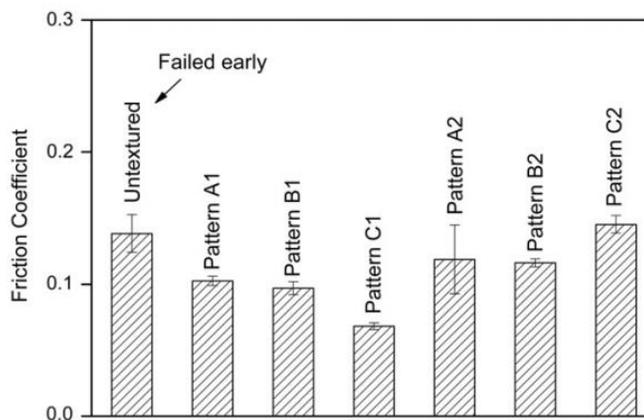
Figure 2.3: Comparison of friction coefficient for all specimen tested under condition Set 1
