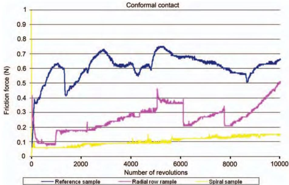
Figure 2.9: Friction force variation with number of revolution under sliding speed of 0.4 m/s
