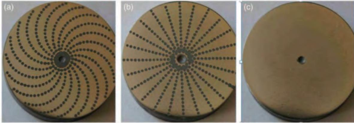
Figure 2.7: Photo of texture disc a) type 1, b) type 2, c) untextured
