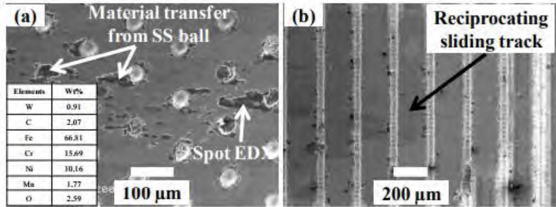
Figure 2.12: SEM images of a) dimples b) grooves
