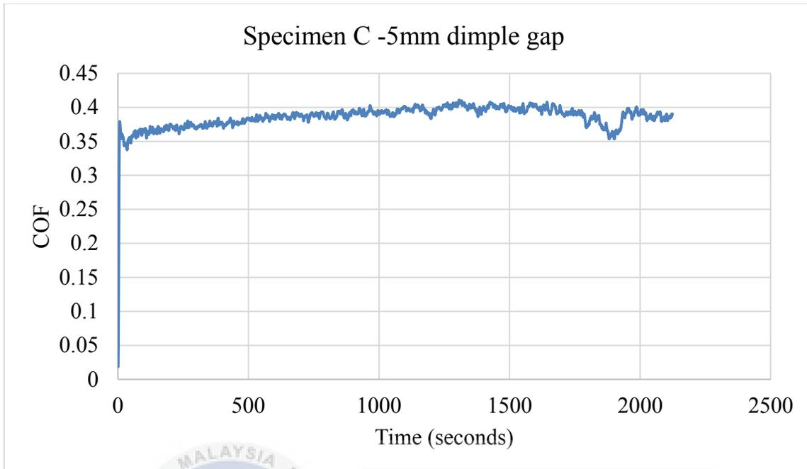
Figure 4.3: The effect of 5mm dimple gap on COF of acrylic disc against stainless steel ball at room temperature
