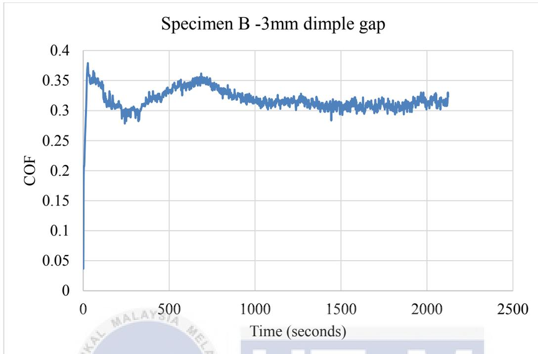
Figure 4.2: The effect of 3mm dimple gap on COF of acrylic disc against stainless steel ball at room temperature
