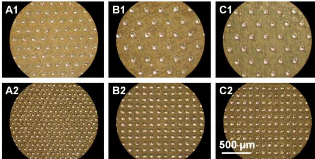
Figure 2.1: Optical images of the unpolished surface texture patterns
