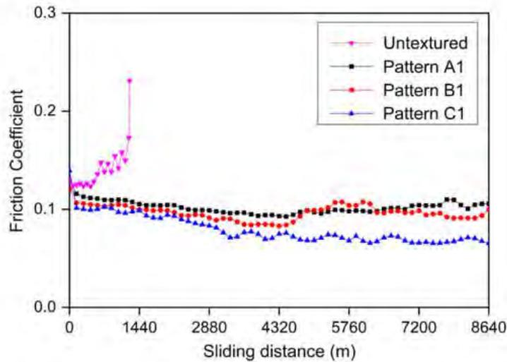
Figure 2.2: Friction coefficient of untextured pattern A1, B1 and C1 under wear test
