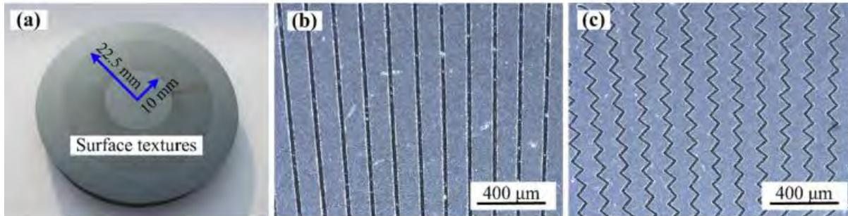
Figure 2.17: Photo of sample and texture pattern a) textured ceramic disc, b) linear grooves, c) wavy grooves
