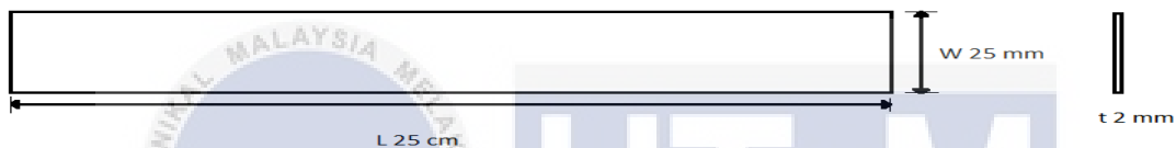
Figure 3.4: Dimensions of AA 6061 specimen for initial tensile test
