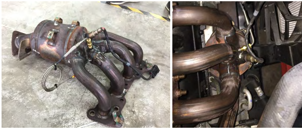
Figure 24 Thermocouple Placement at the Manifold
