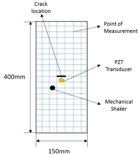
Figure 3.11: The total point of measurement is 114 which included 19 points (top to bottom) in vertical line and each horizontal line have 6 points (left to right)
