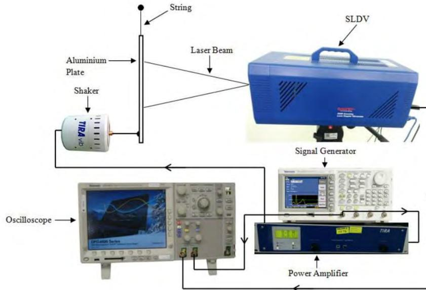
Figure 3.8: Schematic diagram of the experiment setup for experiment modal analysis
