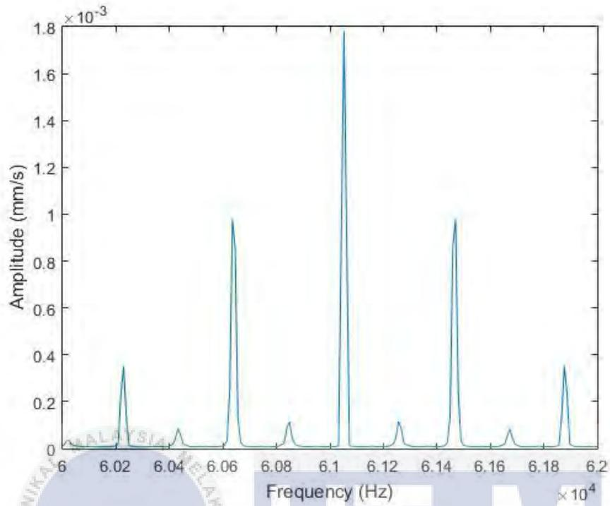
Figure 4.17: Frequency spectrum around 60k Hz for fourth natural frequency (203Hz)
