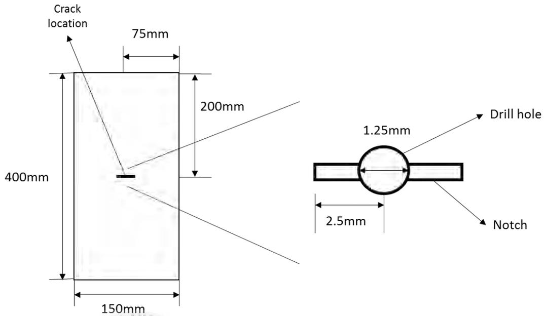
Figure 3.4: Schematic diagram of the aluminum plate and the dimension for drill hole and notch length.
