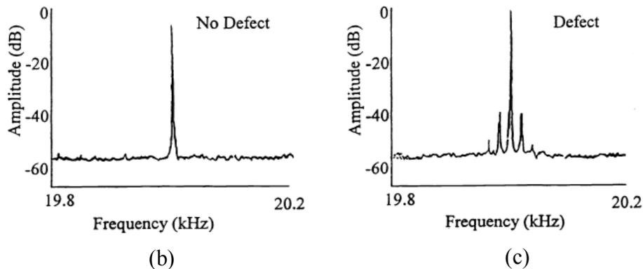
Figure 2.4: (a) Example of signal without crack and (b) Example of signal with crack.
