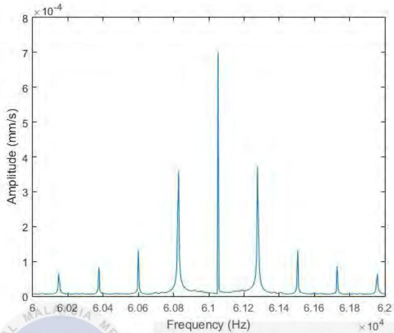
Figure 4.10: Frequency spectrum around 60k Hz for second natural frequency (111Hz)
