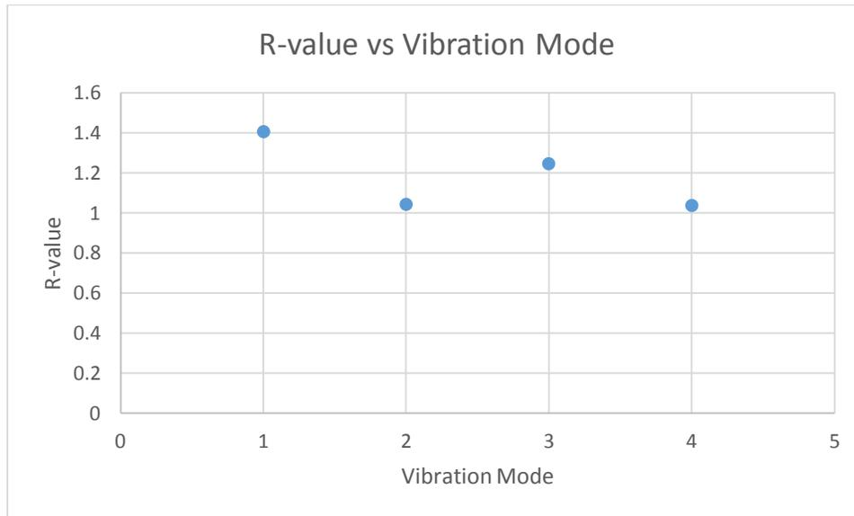
Figure 4.13: R-value verse vibration mode for crack location above middle
