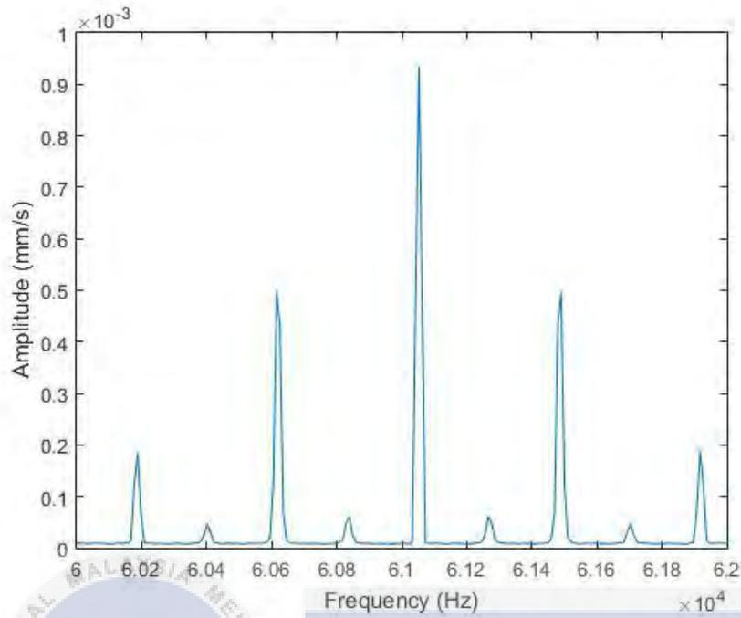
Figure 4.7: Frequency spectrum around 60k Hz for fourth natural frequency (212Hz)
