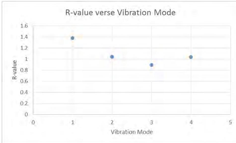
Figure 4.18: R-value verse vibration mode for crack location at edge
