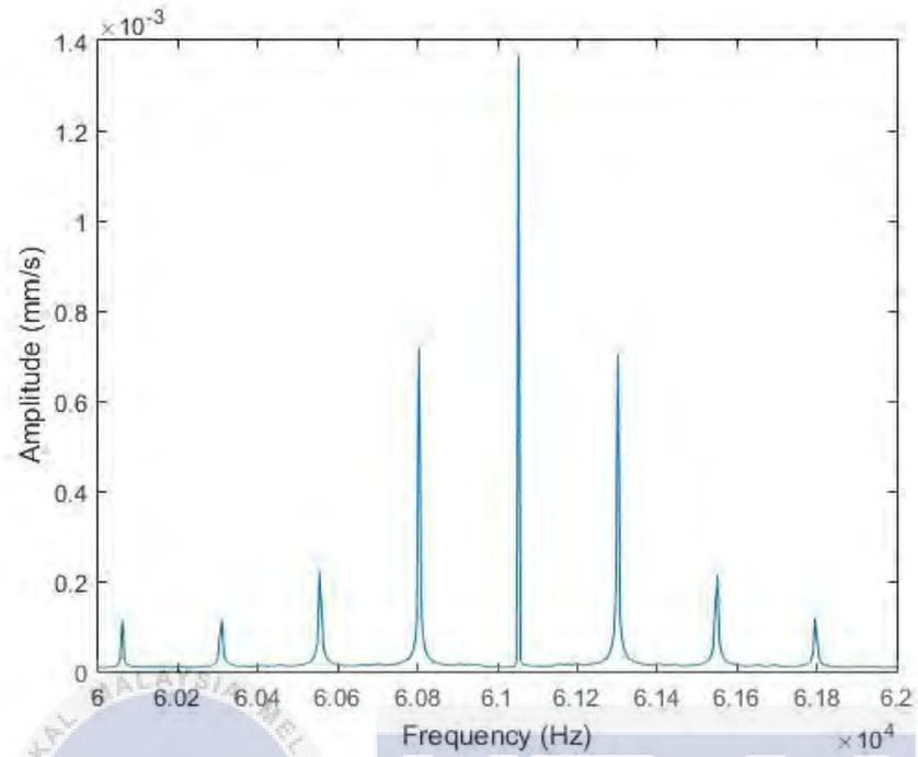
Figure 4.15: Frequency spectrum around 60k Hz for second natural frequency (122Hz)
