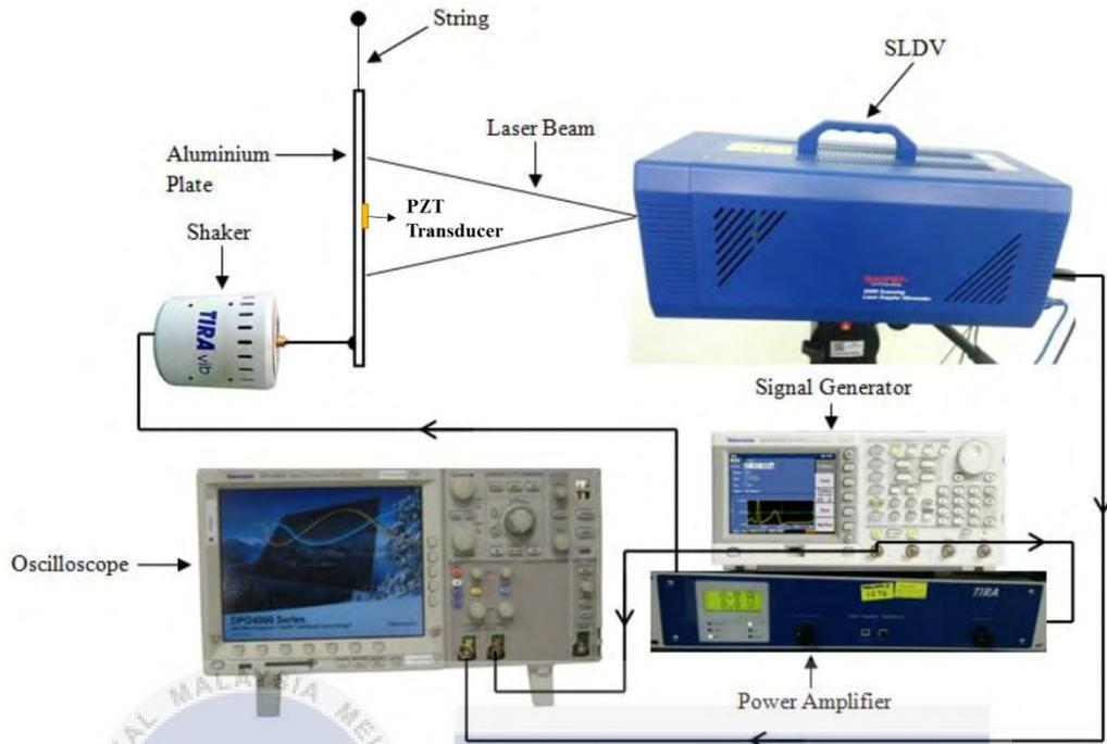
Figure 3.9: Schematic diagram of the experiment setup for vibro-acoustics method (VAM)
