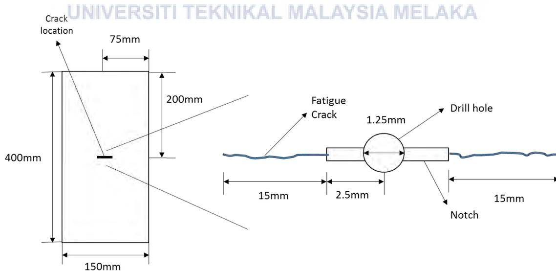
Figure 3.7: Schematic diagram of fatigue crack size
