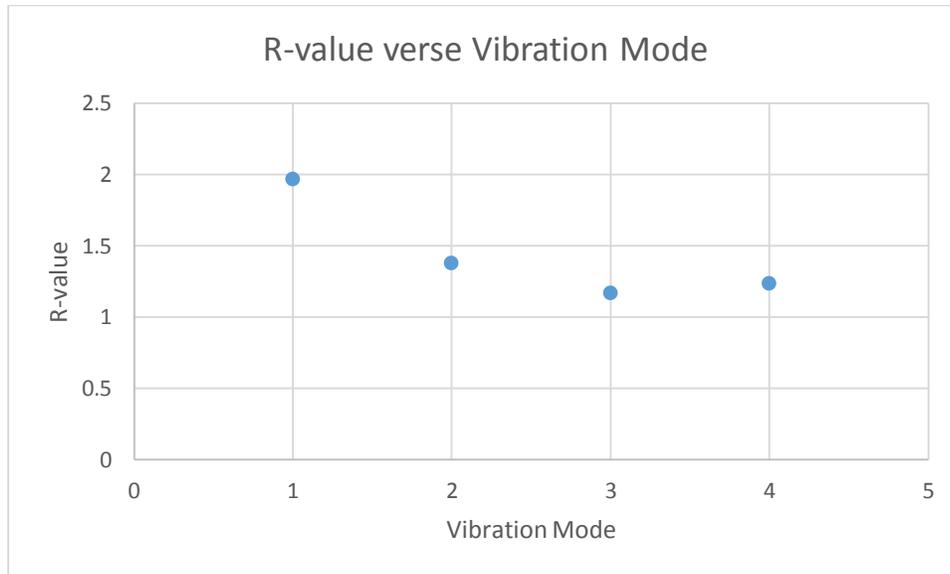
Figure 4.8: R-value verse vibration mode for crack location at middle
