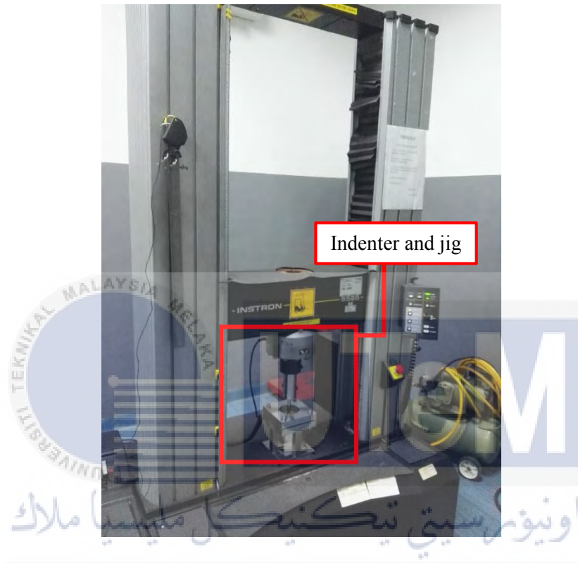
Figure 3.9: Universal Testing Machine Instron 5585 machine for Quasi-static indentation test
