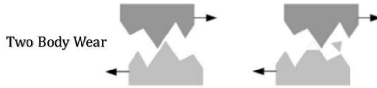
Figure 2.2 Two body abrasive wear (Kopeliovich, 2017)
