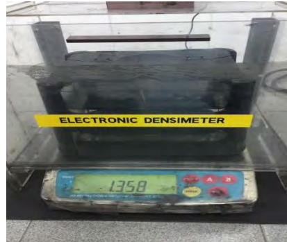
Figure 3.9: Electronic Densimeter for Measuring Density of PALF Samples
