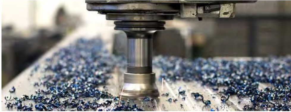
Figure 2.5: Subtractive Manufacturing – Milling process.
