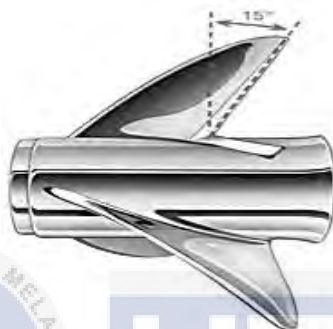
(b) 15 degree rake angle. (Scott Reichow, 2011)
