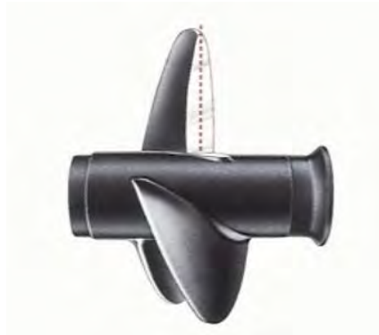
(a) 0 degree rake angle. (Scott Reichow, 2011)
