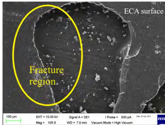
Figure 4.22: SEM micrograph showing fractured region of the ECA with 5 wt.% MWCNT filler loading (low aspect ratio top view of sample).
