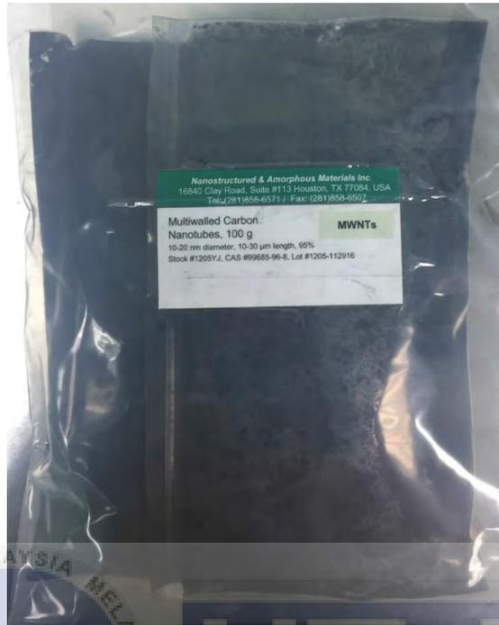
Figure 3.4: Nano Amor MWCNT with 1750 aspect ratio
