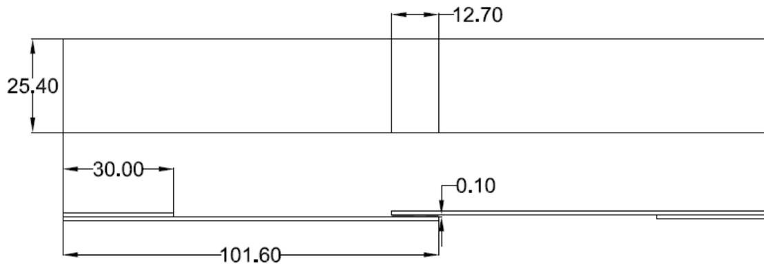
Figure 3.9: Drawing of mechanical specimen
