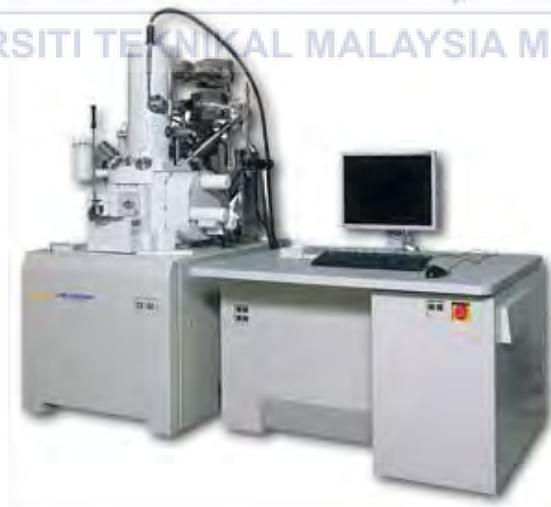
Figure 3.15: Scanning Electron Microscope (SEM)
