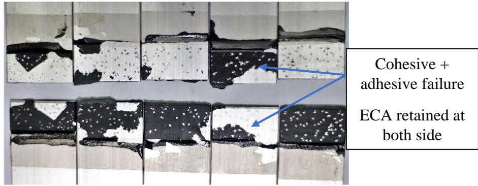
Figure 4.9: 6 wt.% low aspect ratio MWCNT ECA mechanical test samples.
