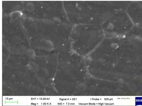
Figure 4.18: SEM micrograph showing the fractured surface of ECA containing 5 wt.% of MWCNT (low aspect ratio) at x1,000 (top view of sample).
