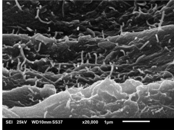
Figure 4.15: 7 wt.% high aspect ratio MWCNT distribution in ECA image obtained using SEM.
