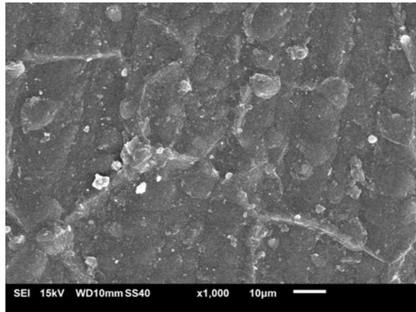
Figure 4.16: SEM micrograph showing the fractured surface of ECA containing 5 wt.% of MWCNT (high aspect ratio) at x1,000 (top view of sample).
