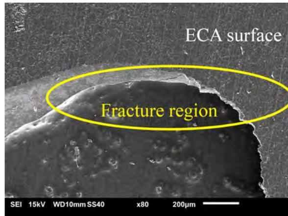
Figure 4.20: SEM micrograph showing fractured region of the ECA with 5 wt.% MWCNT filler loading (high aspect ratio top view of sample).
