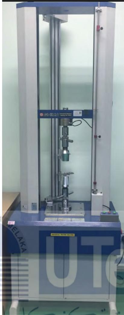
Figure 3.13: Universal testing machine for lap shear test
