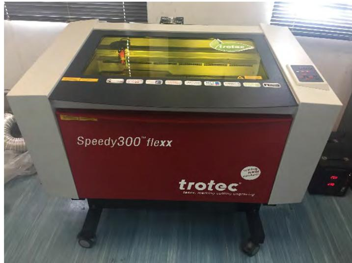
Figure 3.12: Acrylic laser cutting machine.
