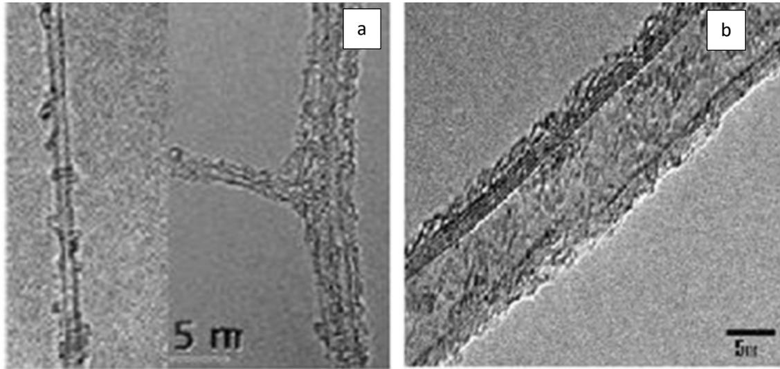
Figure 2.6: Transmission Electron Microscope (TEM) images of (a) SWCNT (b) MWCNT [27].
