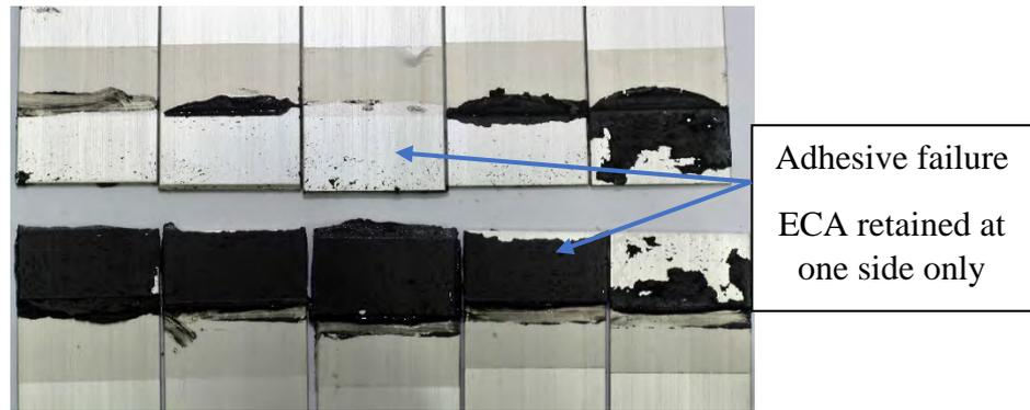
Figure 4.7: 7 wt.% high aspect ratio MWCNT ECA mechanical test samples.
