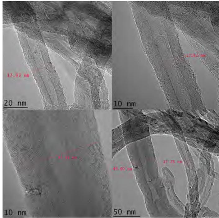
Figure 4.12: TEM image showing the high aspect ratio MWCNT diameter.
