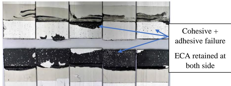
Figure 4.5: 5 wt.% high aspect ratio MWCNT ECA mechanical test samples.
