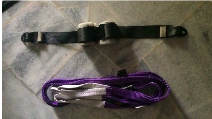
Figure 4.1: Sling tow and seatbelt retractor
