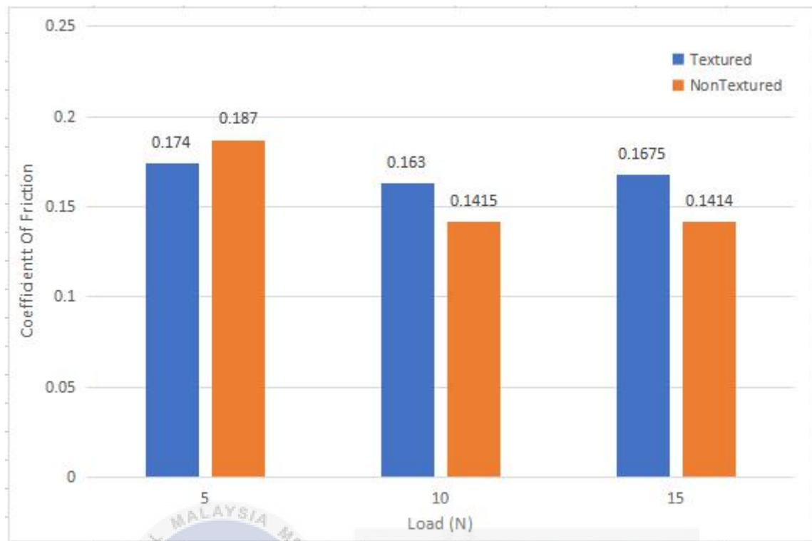
Figure 4.16: Coefficient of friction against load for 200rpm
