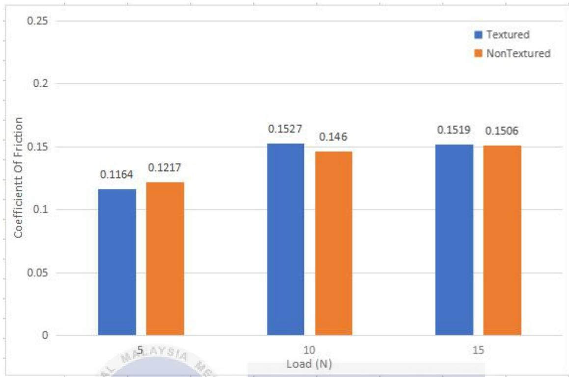
Figure 4.15: Coefficient of friction against load for 150rpm
