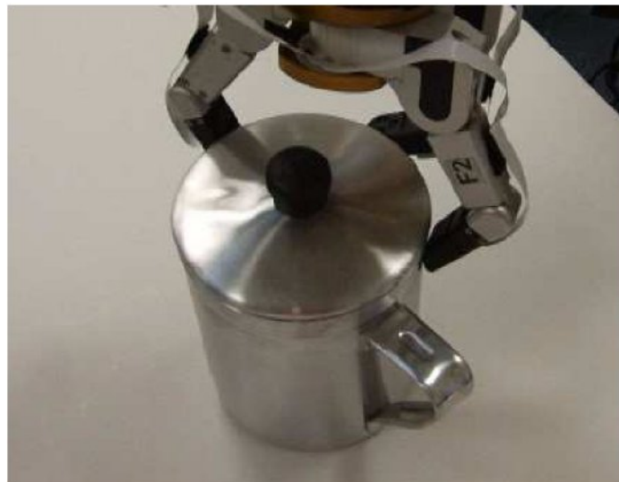
Figure 2.5 shows the effect of grasping proximity sensor gripper on shiny object.
