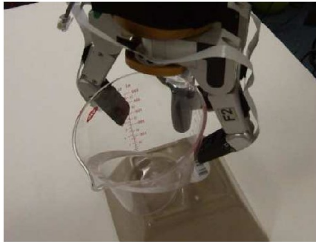
Figure 2.6 shows the effect of grasping proximity sensor gripper on transparent glass.
