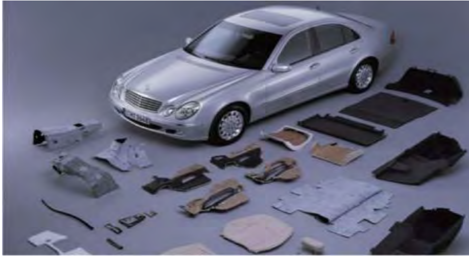
Figure 2.4: Mercedes Benz automotive parts fabricated by natural fibres (Monteiro et al., 2010)
