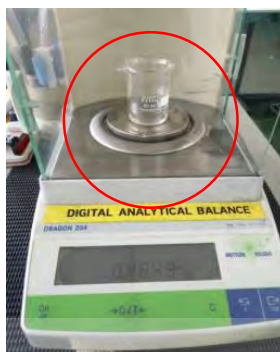
Figure 3.2 Beaker positioned on the centre of pan
