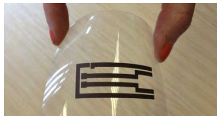
Figure 1.1 Printed conductive ink (Savastano, "Conductive Inks Drive Growth in Flexible and Printed Electronics ", 2015)
