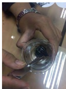
Figure 3.9: Mixing process of resin, hardener and electrically conductive ink
