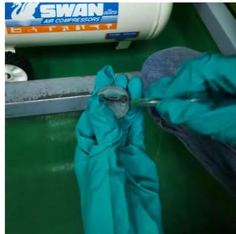
Figure 3.34: Etching process of solder alloy.
