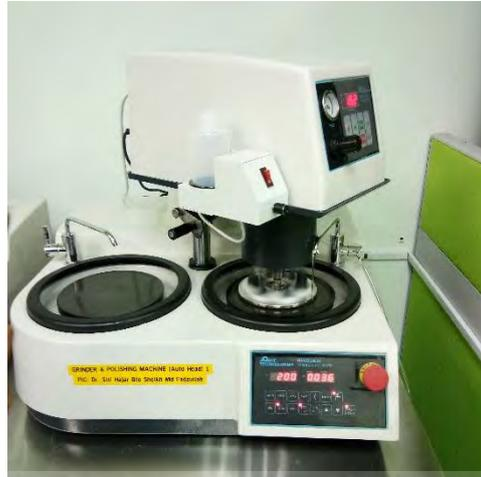
Figure 3.30: Grinder and polishing machine.
