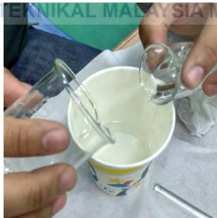
Figure 3.25: Mixing resin and hardener process.
