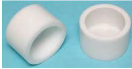
Figure 3.24: Cold mounting silicone rubber mold.
