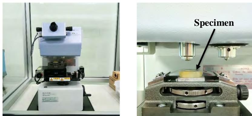
Figure 3.39: Nano Indentation measurement device.
