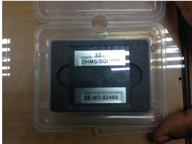
Figure 3.37: Calibration stage tool.
