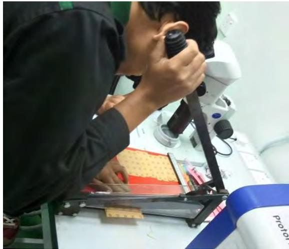
Figure 3.12: Cutting positive board process using board cutter.
