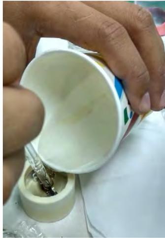
Figure 3.27: Pouring cold mounting mixture into the mold.
