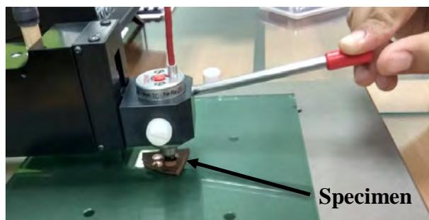
Figure 3.38: Electrical resistivity measurement using Four Point Probe.
