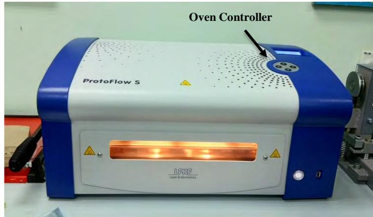
Figure 3.14: Reflow oven machine
