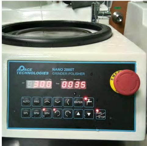
Figure 3.31: Grinder and polisher machine controller.
