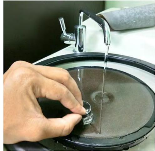
Figure 3.32: Grinding process.
