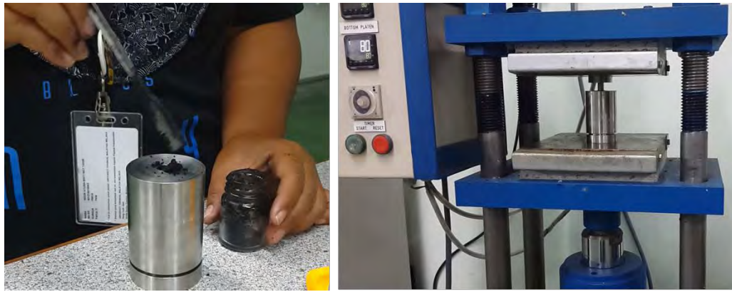
Figure 3.5 : Preparing the compaction process by inserting the slurry composite the mould and compaction process
