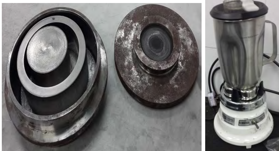
Figure 4.6 : Grinding bowl with heavy duty blender
