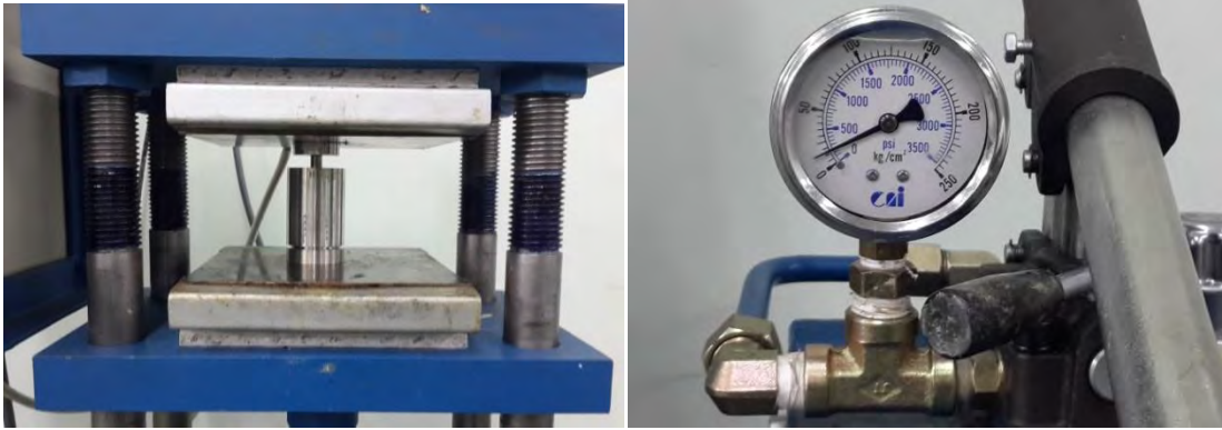
Figure 4.9 : Compaction process with pressure of 150 psi
