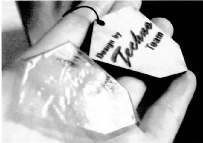
Figure 7.35(b) Successful vacuum formed product.
