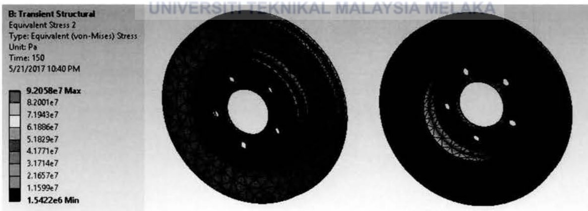
Figure 5.22: Equivalent (von-Mises) stress at 150 seconds
